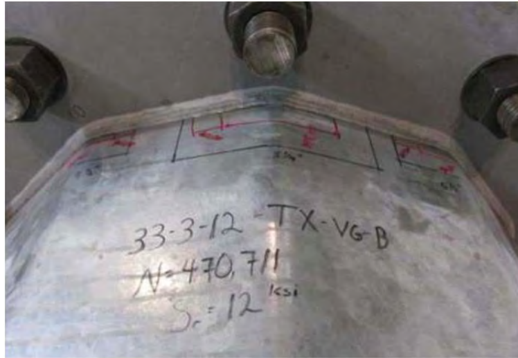
Figure 7.15: Specimen 33-3-12-TX-VG-B after Fatigue Testing
