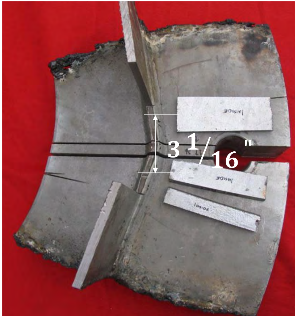
Figure 7.6: View of Bend 5 after Sectioning. Length of Observed Initial Crack is Labeled
