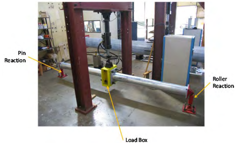
Figure 2.3: Portal Loading Frame High-mast and Mast Arm Tests
