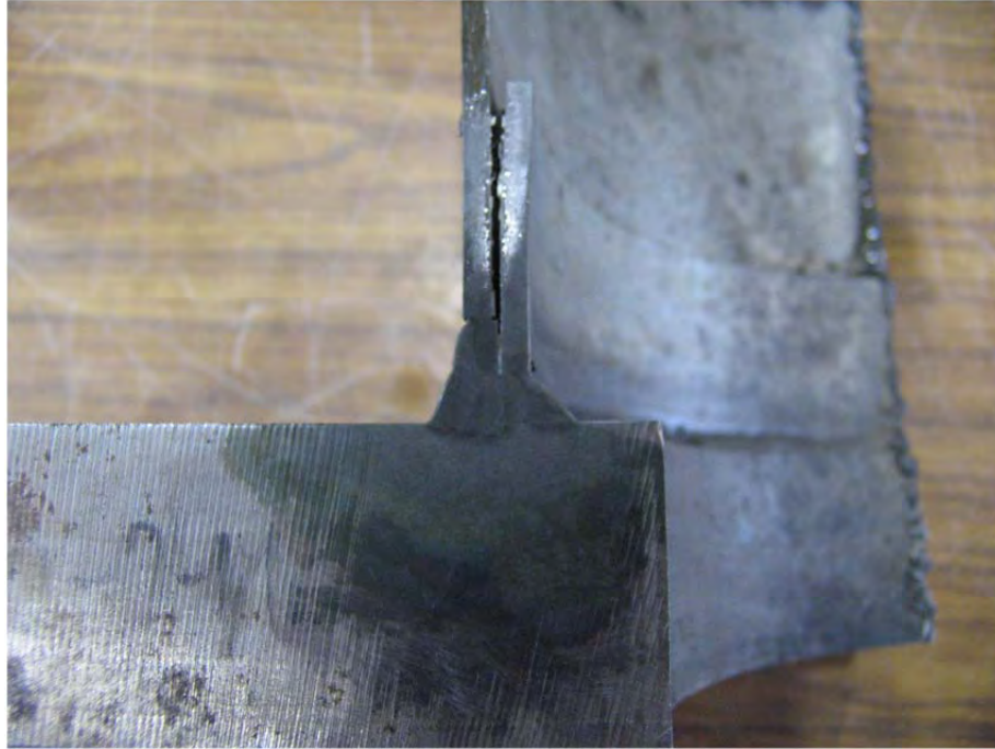
Figure 3.2: Cross Section of a Typical Full Penetration Connection
