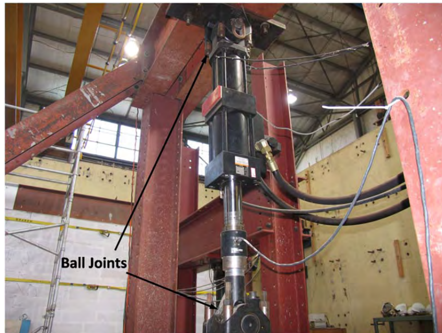
Figure 2.4: MTS 55-kip Hydraulic Actuator
