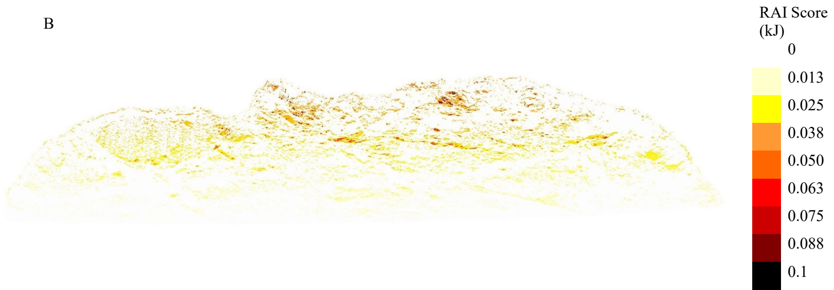
Figure 4.10 RAI classes (A) and RAI scores (B) for the 2018 scan of the study slope at MP 241 on the George Parks Highway near Glitter Gulch, Alaska.
