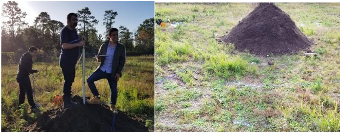
Figure 3-13. Magnetic extensometer readings after first loading stage and soil volume control lines
