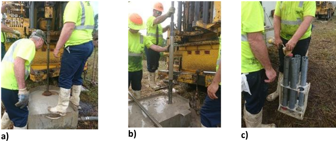
Figure 3-10. Sampling process of the Shelby tubes: (a) drilling, (b) extraction, and (c) wax sealing
