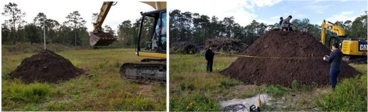
Figure 3-16. Measurements of conical shape taken at different loading stages
