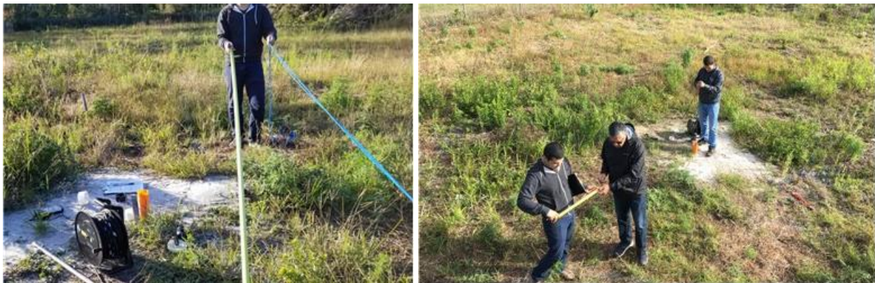
Figure 3-15. Inclinometer reading station at an intermediate conical load stage
