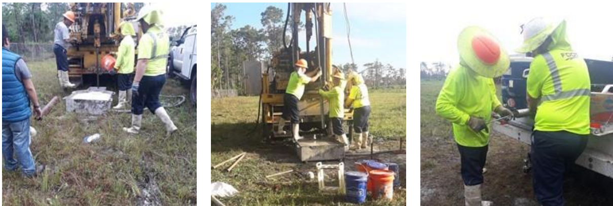
Figure 3-10. Sampling process of the Shelby tubes: (a) drilling, (b) extraction, and (c) wax sealing
