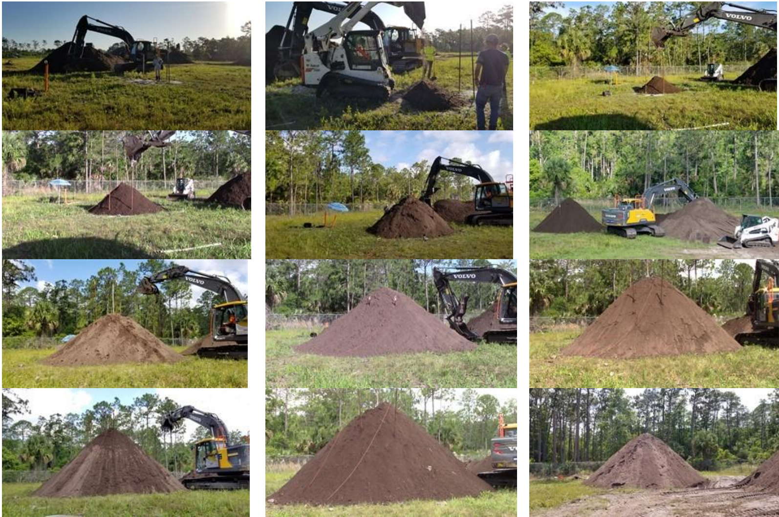
Figure 3-18 b. Pictures of conical load testing sequence for Cone 2. Pictures taken on May 10, 2019
