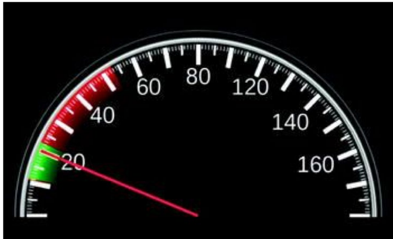
Figure 1.1: A GLOSA interface for motor vehicles. The green band moves to place the driver in a green wave.
