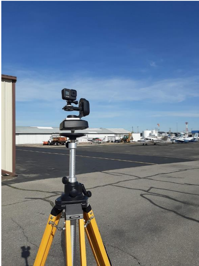
Figure 9 GoPro Hero 8 camera setup
