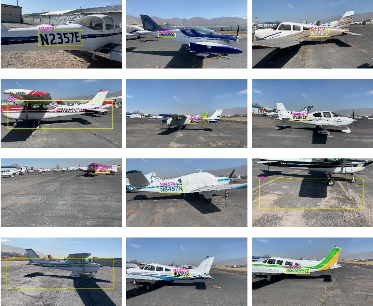
Figure 24 TRD (yellow box) and OCR (pink font) results on sample photos from aircraft parked in the apron area
