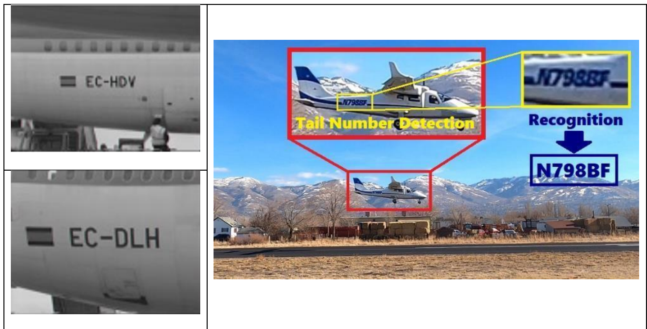
Figure 4 Left: Images from airliners’ tail numbers (Molina et al., 2002), Right: A video frame of an aircraft in motion (landing, camera layout 1)
