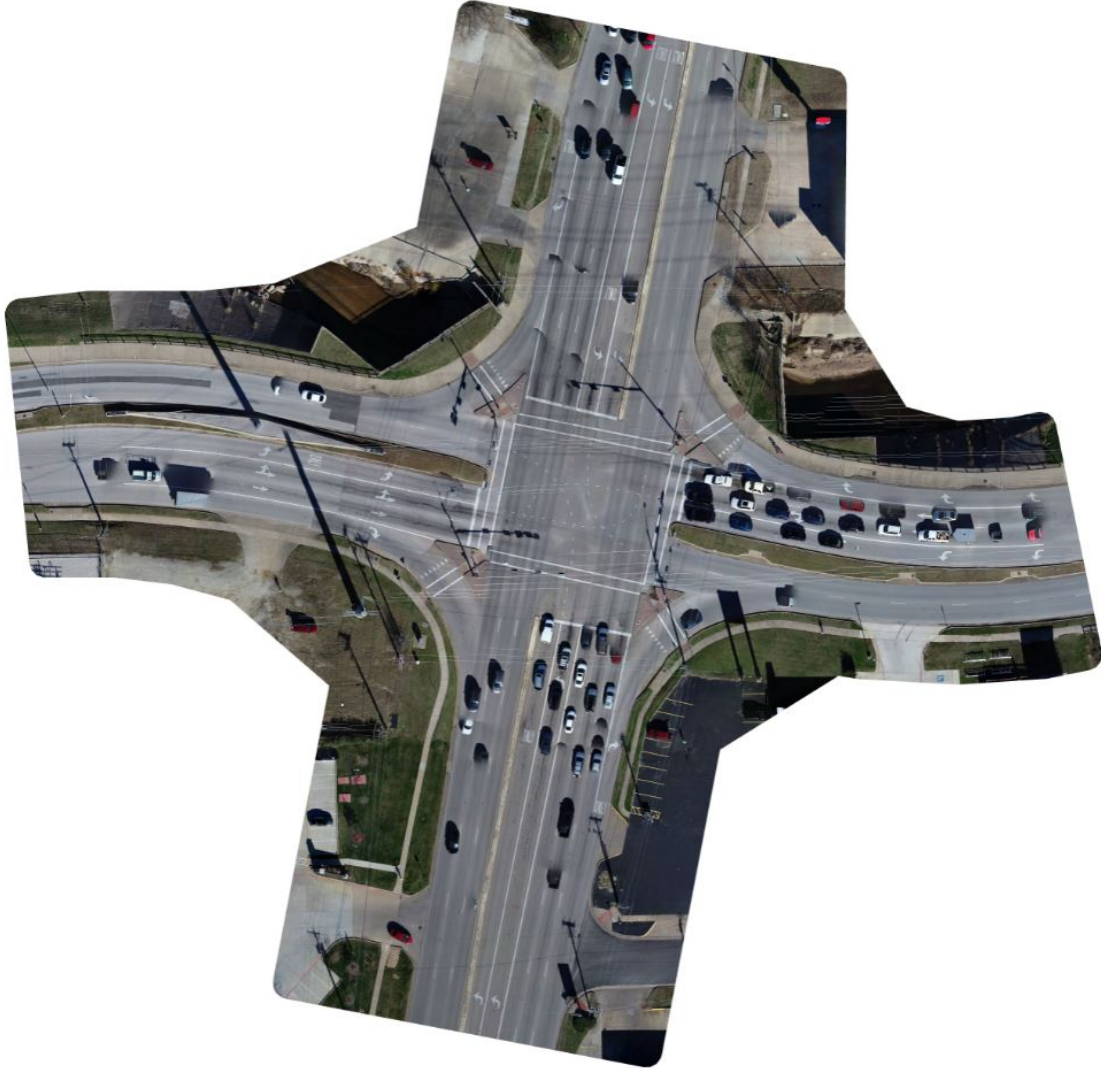
Figure 5. Orthomosaic of the Tyler intersection generated from the aerial images
