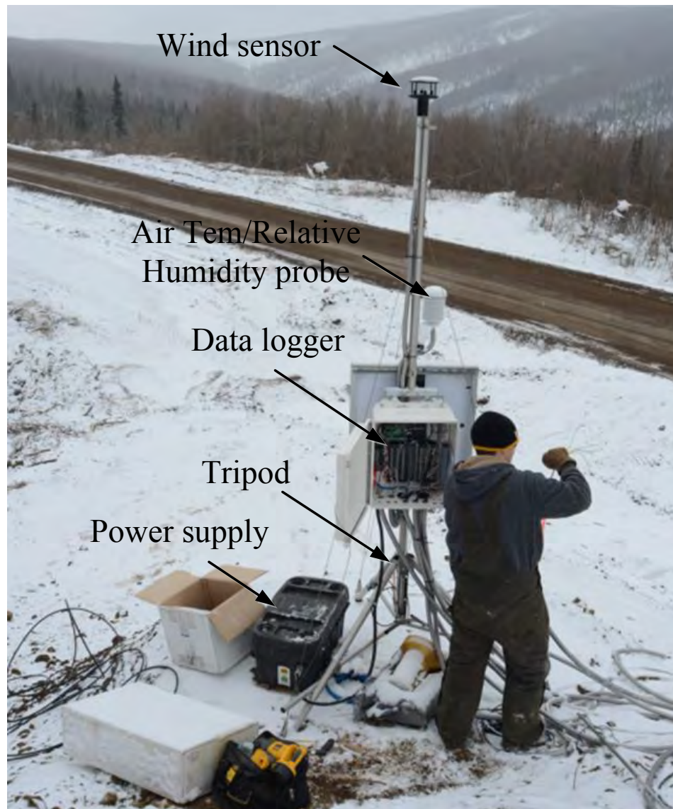
Figure 5.4 Data collection station
