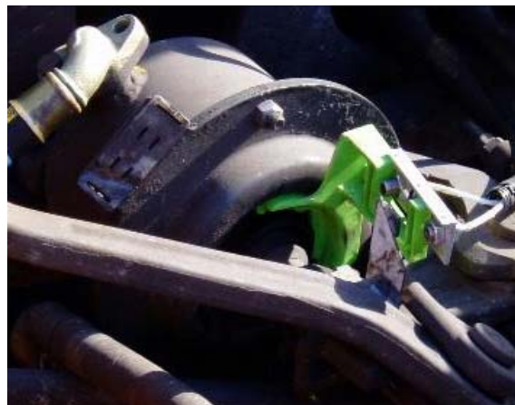
Figure 1. Brake piston travel sensor arrangement.
