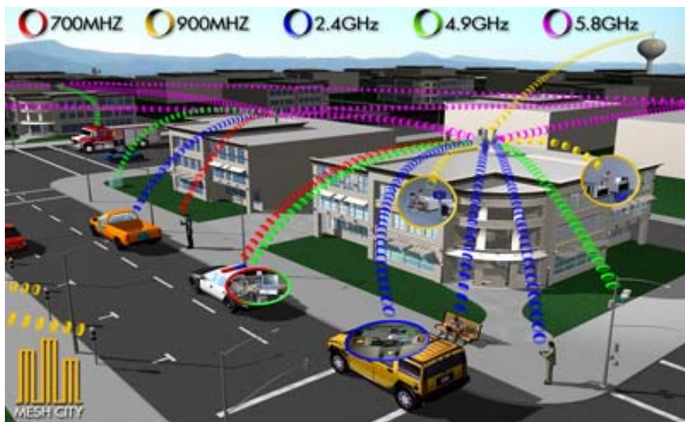
Figure 10: Mesh city's frequencies of operation (Courtesy Mesh City).
