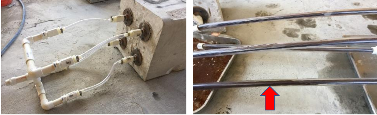
Figure 4-17: Manifold attached to the back of the specimen (left); Clear tubing filled with WD-40 (right).
