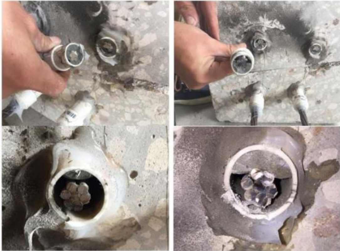
Figure 4-5: Tendon 1 with no water injection (top left); Tendon 2 with 10-cc water injection (top right); Tendon 3 with 25-cc water injection (bottom left); Tendon 4 with 50-cc water injection (bottom right).
