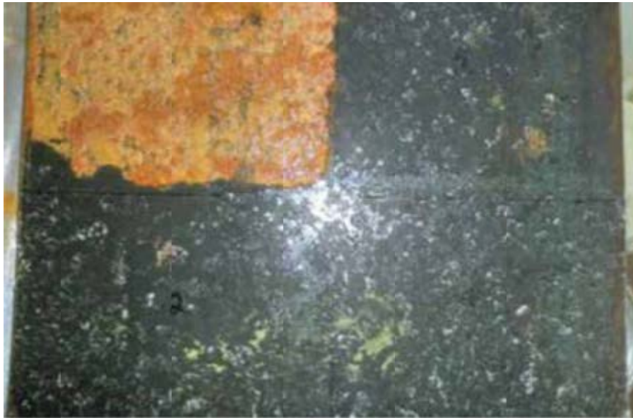
Figure 2-2: Corrosion protection effect of impregnation fluid applied on a steel plate exposed to salt spray test. Compare with untreated upper left portion. 47
