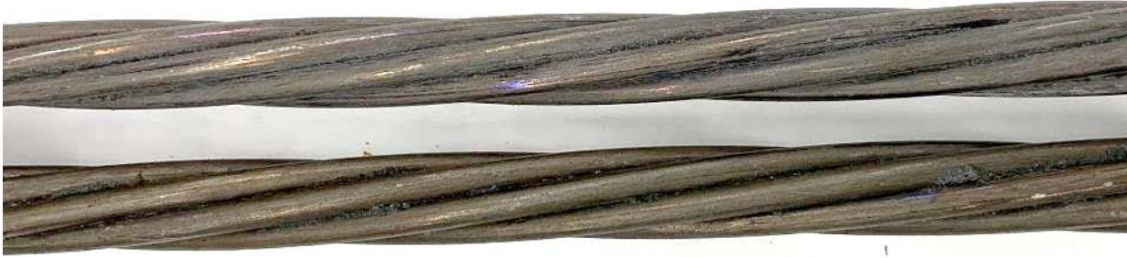
Figure 5-9: The reinforcement extracted from the 1-ft normal tendons. The reinforcement on the top is from the control group and the reinforcement on the bottom is from the impregnated group.
