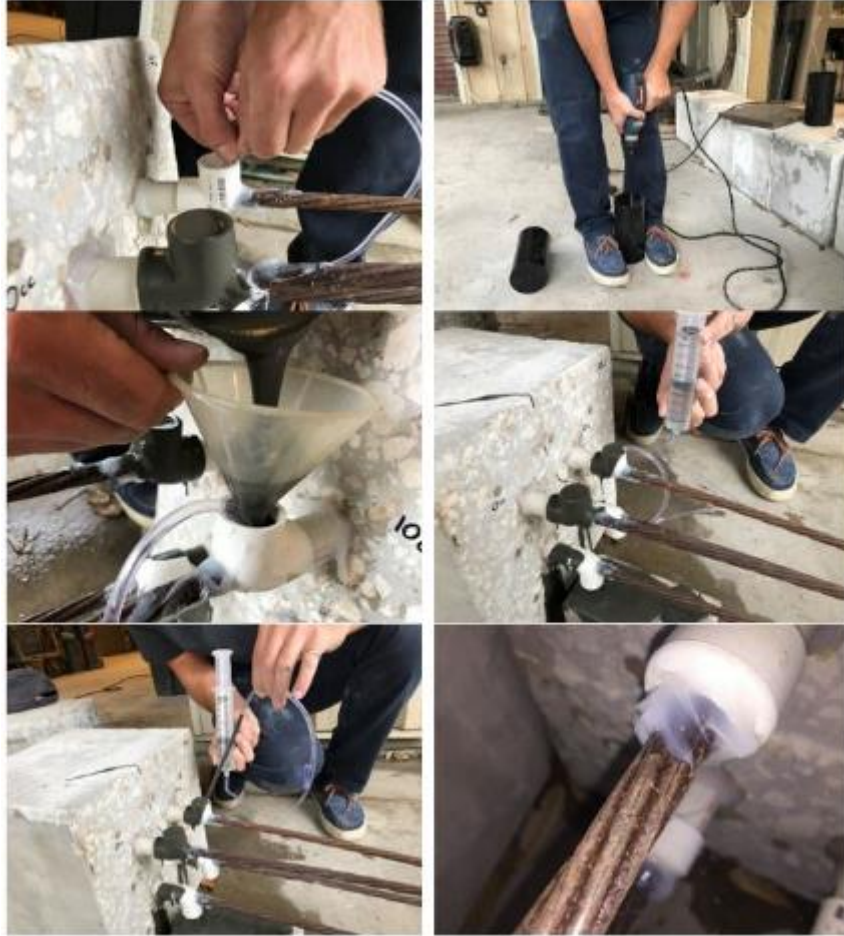
Figure 4-3: Feeding flexible hose into tendon for water injection (top left); Mixing grout in 4x8 concrete cylinder (top right); Pouring grout into funnel to prevent grout spillage (middle left); Removing steel brick to place concrete specimen horizontal and injecting water into tendon (middle right); Extracting flexible hose from tendon (bottom left); Water wicking out of the strand from water injection (bottom right).
