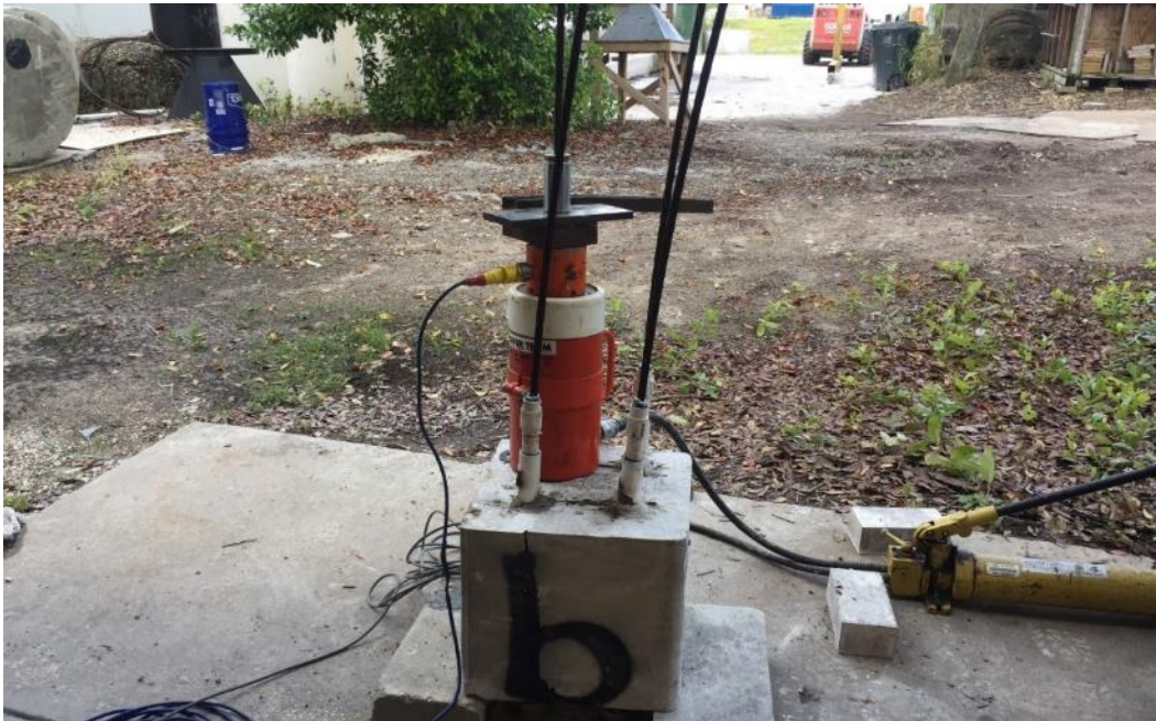
Figure 4-19: Pullout test setup for concrete specimen 9.
