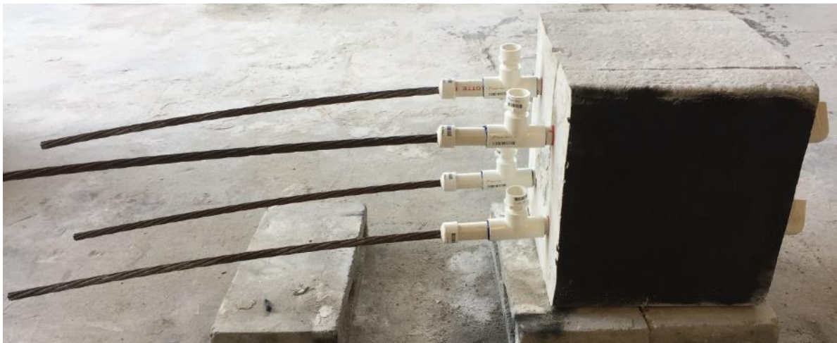
Figure 4-11: Concrete specimen 9 before grout installation.
