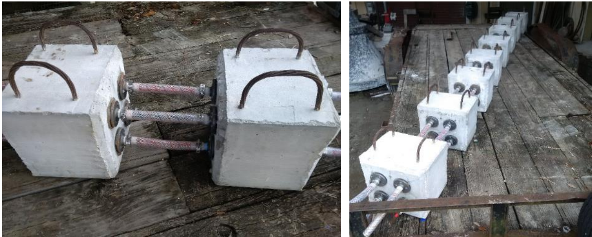
Figure 4-55: Pile segments complete with pipe flanges, barbed hose fittings, and high-pressure hoses to simulate a longer length duct.
