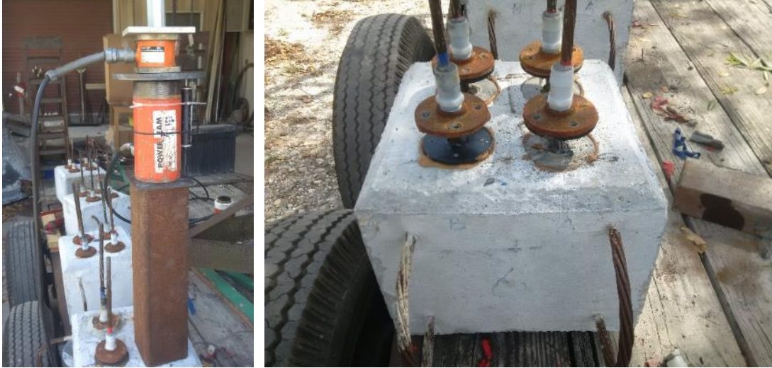
Figure 4-61: Pullout testing (left); flange displaced upward 2 in (right)
