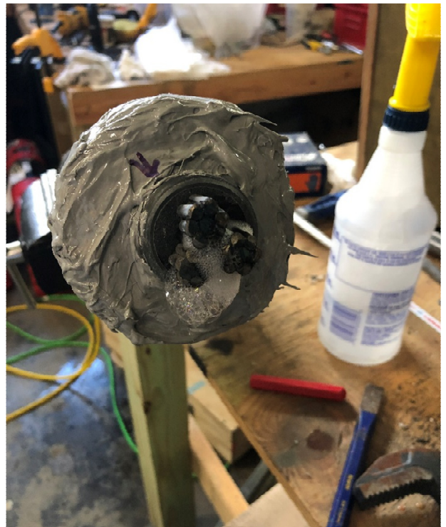
Air testing 3ft Specimen – photo shows bubbles formed by air exiting the interstitial spaces in the tendons.
