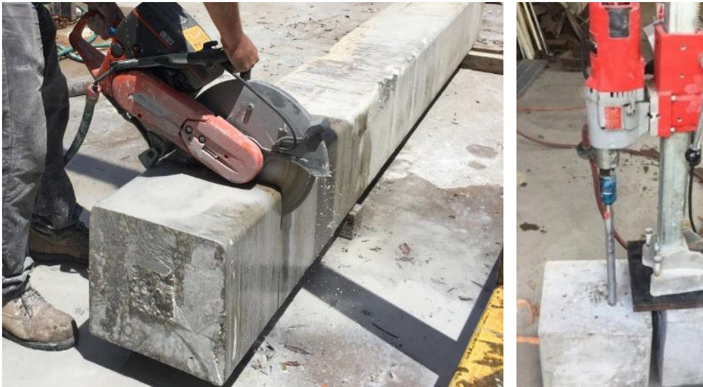
Figure 4-1: Cutting 14-inch square pile for concrete specimens and coring simulate duct corridors into 1ft concrete segments
