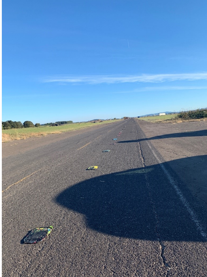
Figure 5.2: Placement of portable traffic analyzers in calibration test
