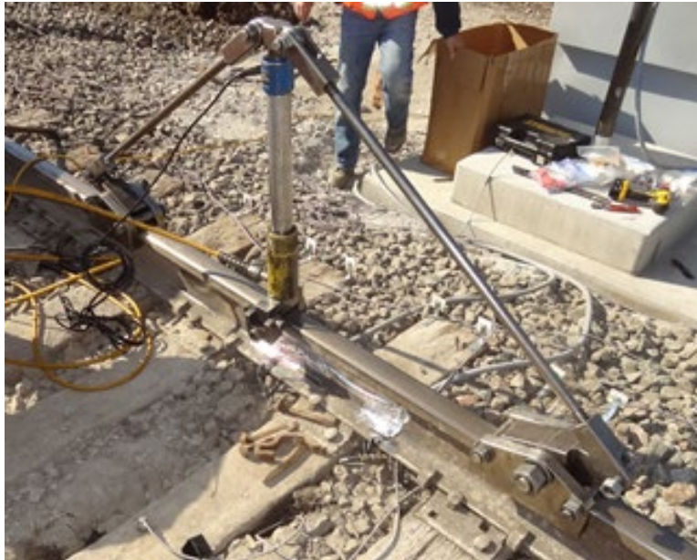
Figure 35. Strain Gauge Calibration Frame
