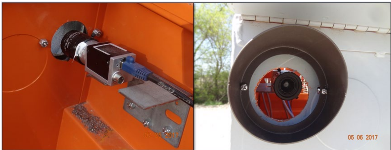
Figure 32. High Frequency Video Camera and Glass Shield
