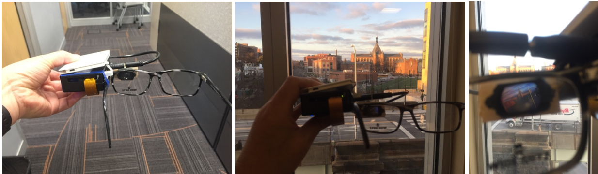
Figure 1. Prototype One: Micro Video HUD (left), test scene of the building in distance (middle) and the HUD view (right)
