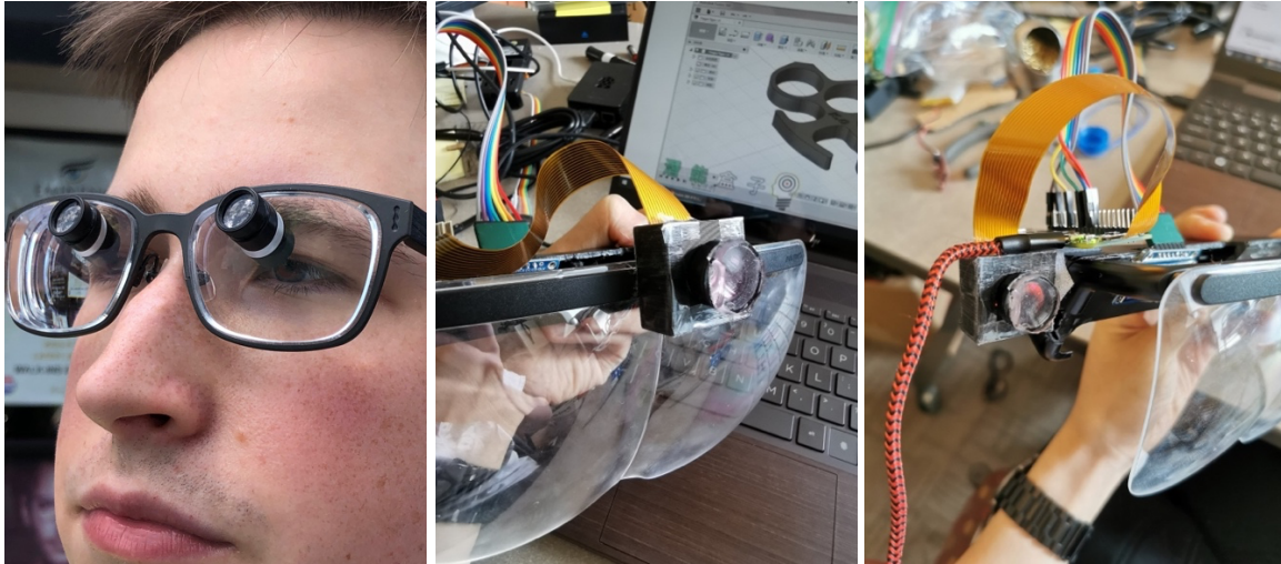
Figure 3. The traditional bioptic telescopic lens (left) and the holographic HUD with telescopic lens (middle and right)
