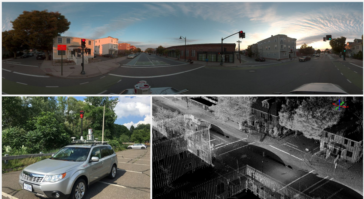
Figure 2.2: LiDAR sensing vehicle (bottom L), video log imagery (top), and point cloud data (bottom R)
