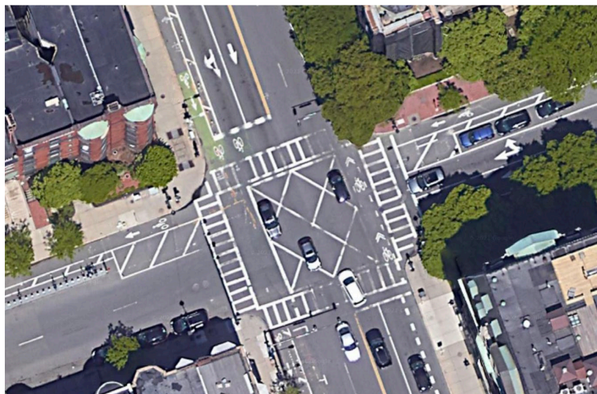
Figure 4.2: Bike box spanning one of two traffic lanes (Massachusetts Ave. at Beacon St., Boston)
