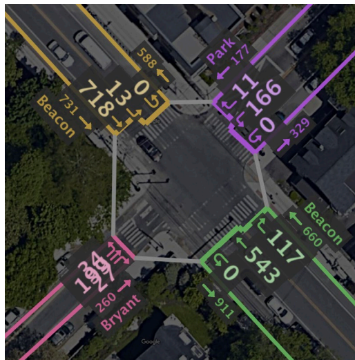
Figure 4.12: Bicycle turning movement counts at Beacon Street and Park Street (11/16/2020 at 3:00 p.m. to 11/17/2020 at 3:45 p.m.)
