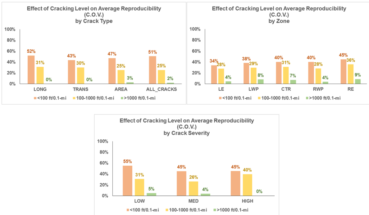
Figure 7.13 Effect of cracking extent on variability in crack survey on the Big Loop.
