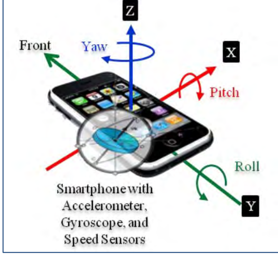
Figure 3.5 Orientation of the mobile device with three angular quantities
