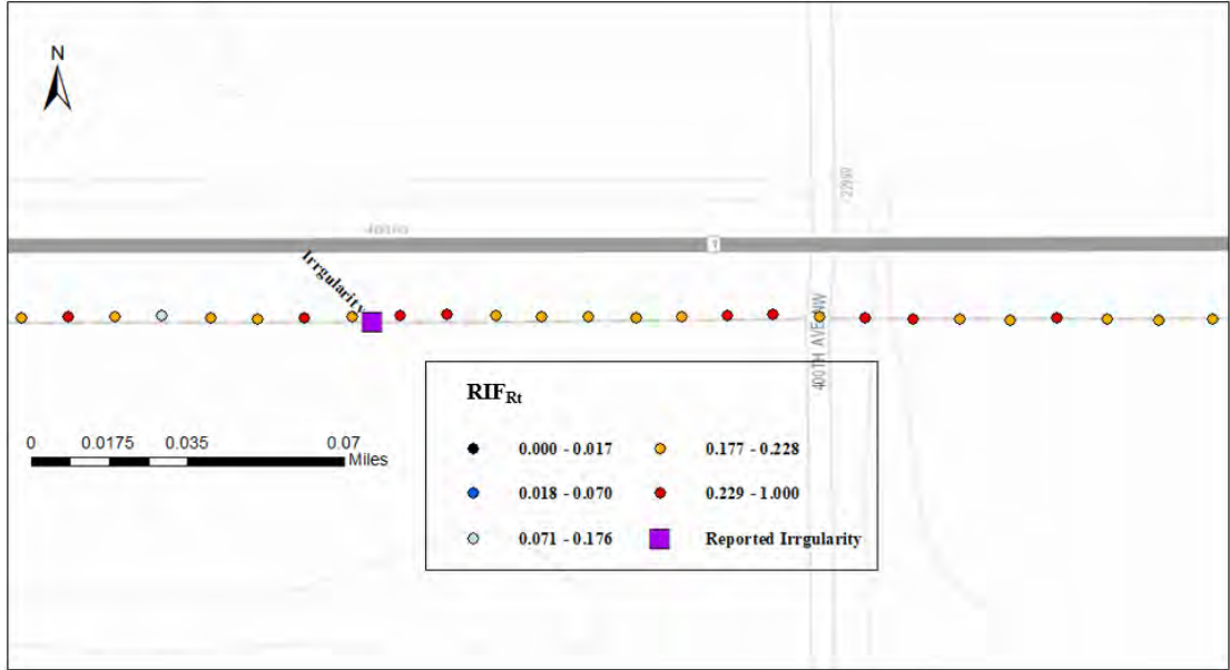
Figure 5.2 A map of PIEs that correspond to severe track irregularity
