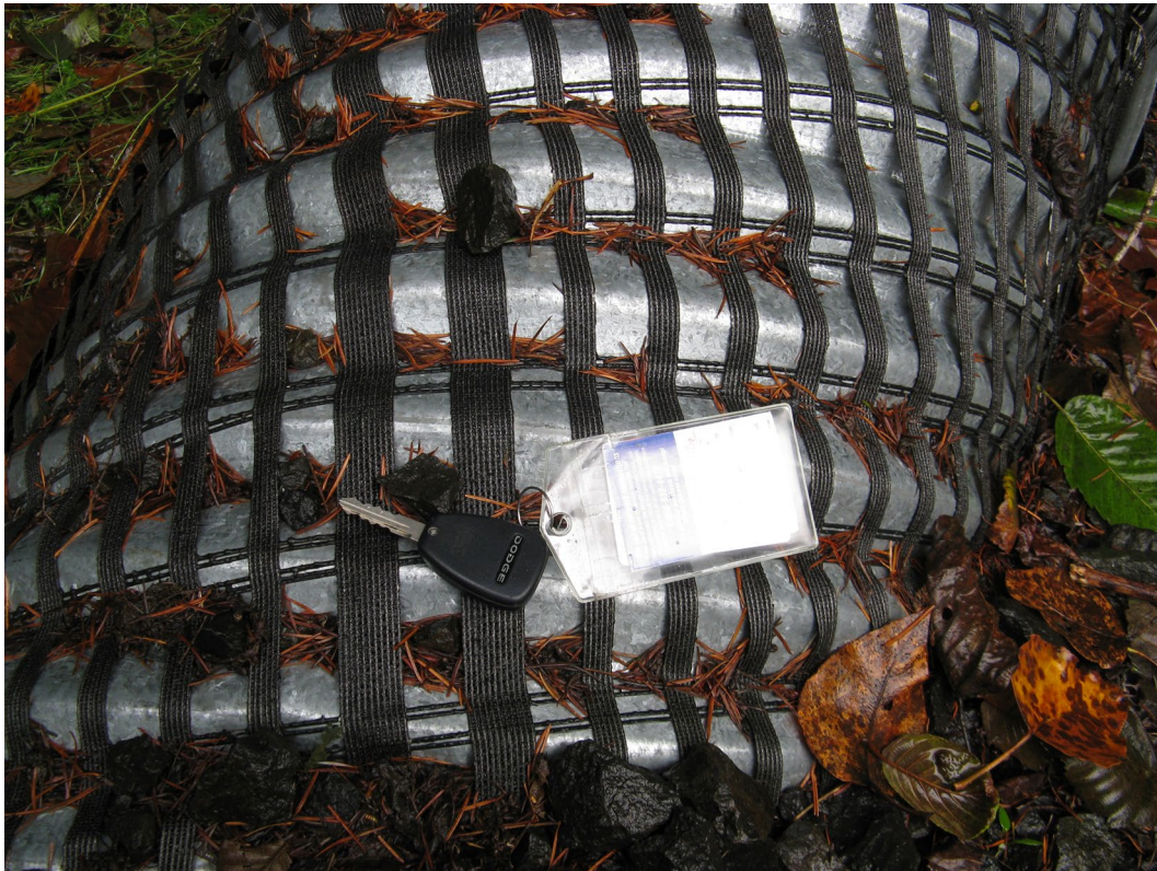
Figure 12: Photo of uniaxial geogrid used on Road 25 repairs in the Gifford Pinchot forest.
