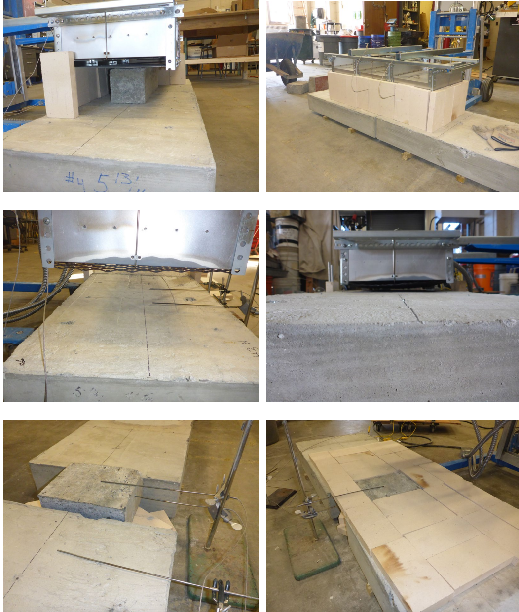
Figure 7.2: Heating chamber configuration (top L and R); direct heating of specimen (center L and R); heating of smaller specimen between two throwaway slabs (bottom L and R)
