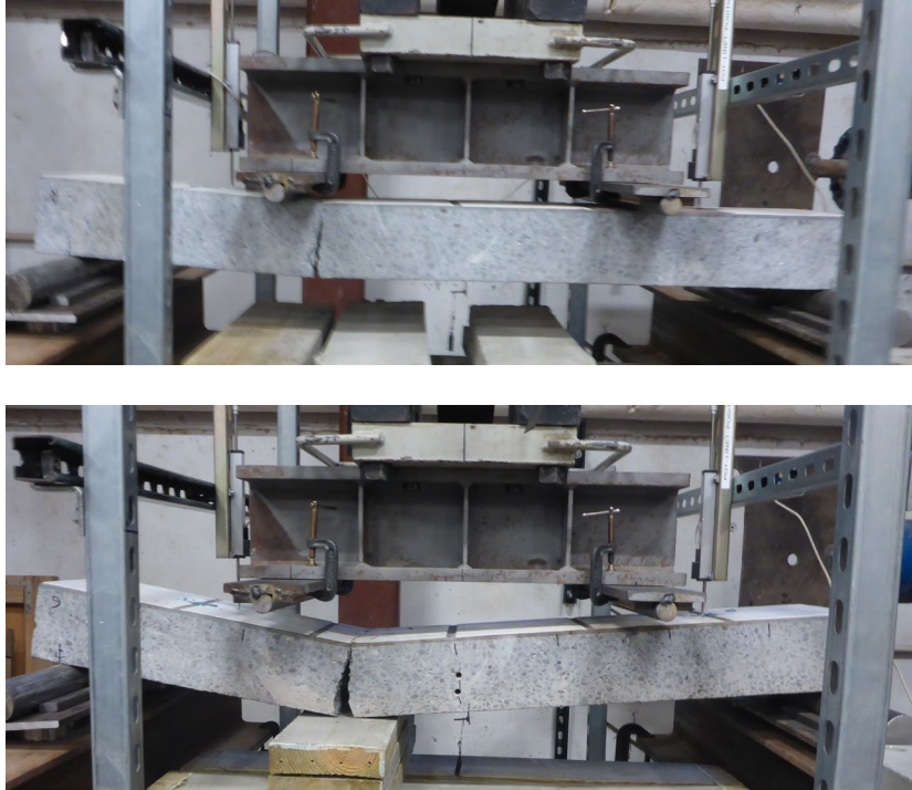
Figure 7.28: Photo of minimally reinforced beam specimens during load testing. Propagation of crack in control specimen during load application (top); after failure of heated specimen (bottom)
