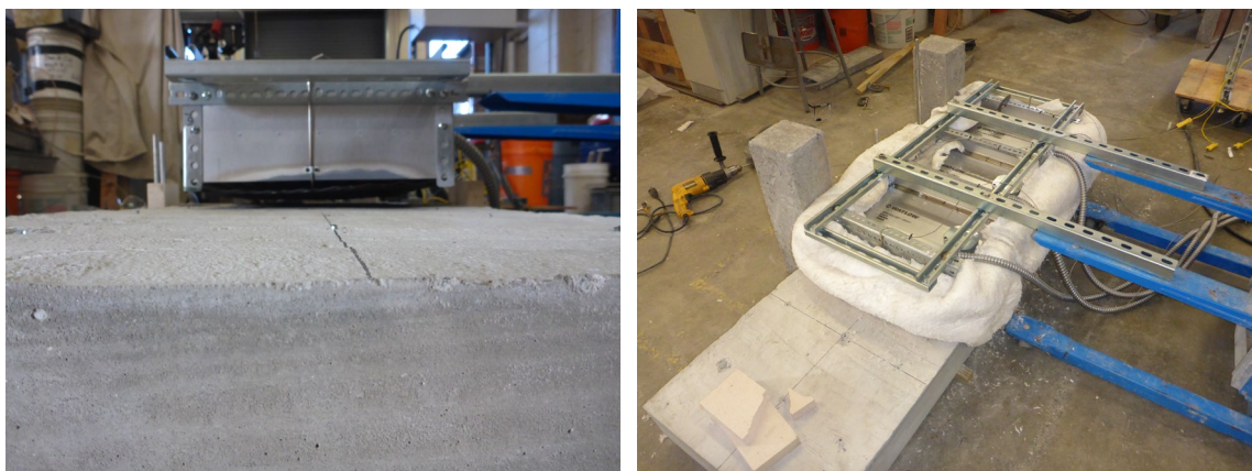
Figure 7.13: Concrete slab heating setup
