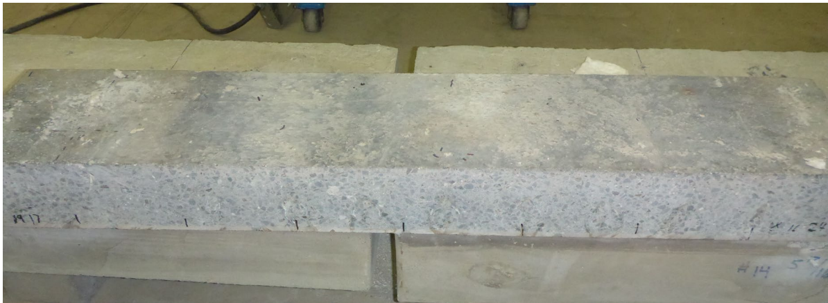
Figure 7.25: Intact minimally reinforced beam specimen after heating
