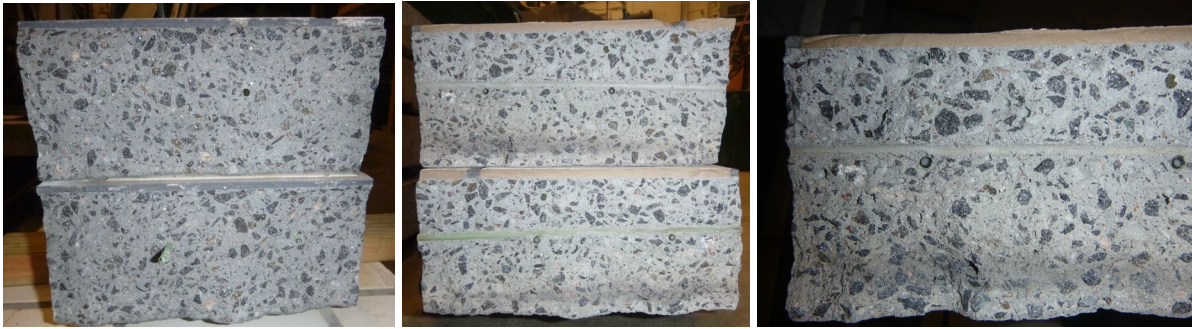
Figure 7.30: Interior visual inspection of heat effects of ruptured specimens: control specimen with consistent color through ruptured sections (L); specimen heated to 600°C specimen (C); closeup of specimen heated to 600°C (R)
