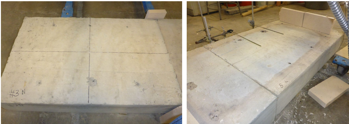
Figure 7.15: Slab before heating (L); whitening after heating to surface temperatures up to 930°C (R)
