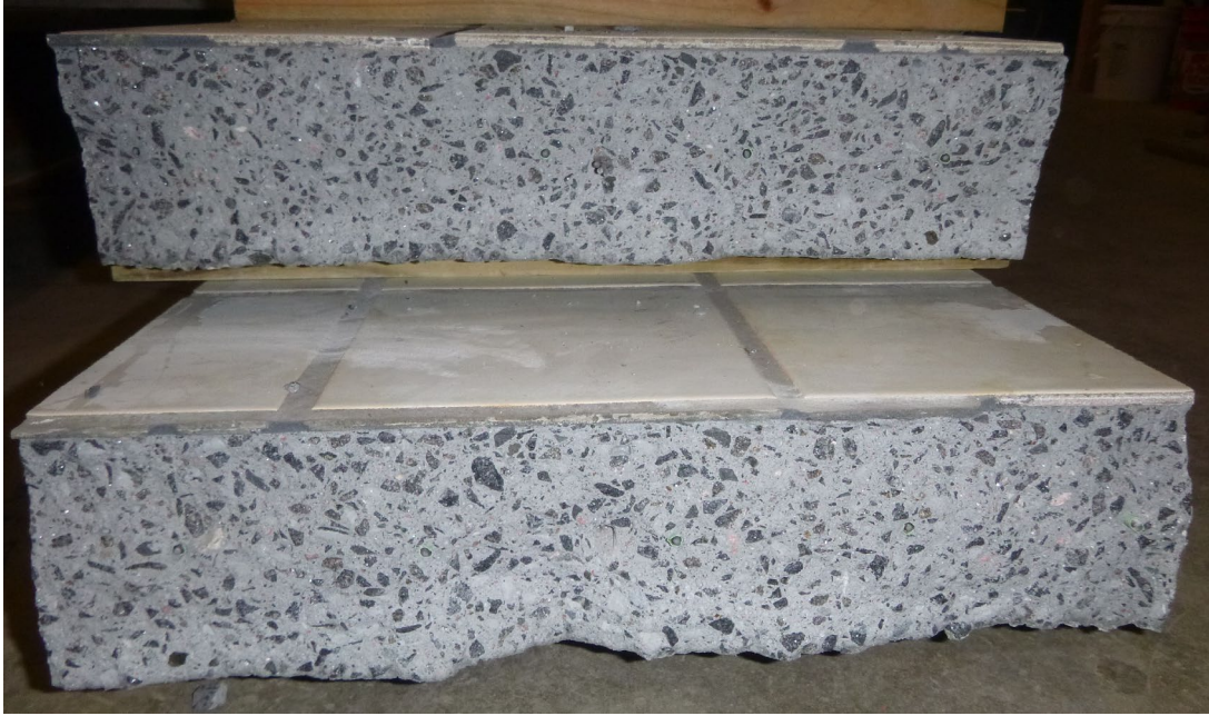
Figure 7.40: Ruptured surface of 300°C heated specimen
