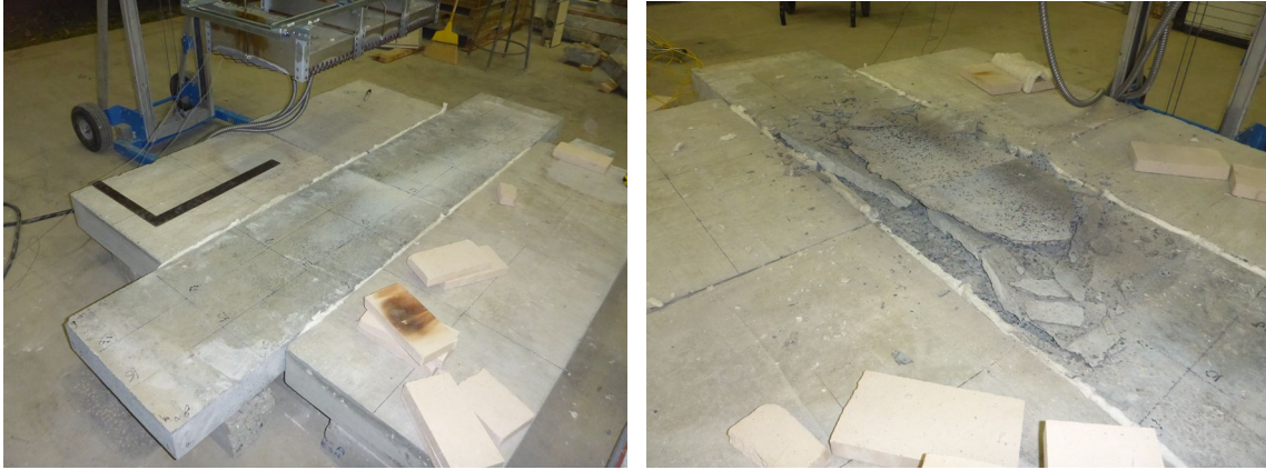
Figure 7.32: Spalling of 600°C beam specimen prior to heating (L), post heating (R)
