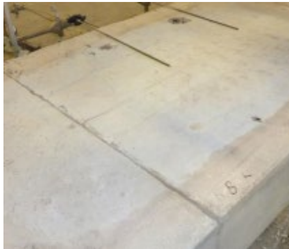
Concrete discoloration at 1000°C (1,832°F)
