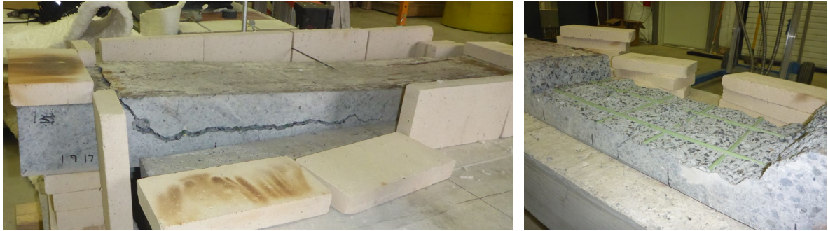
Figure 7.24: Spalled minimally reinforced beam specimen after heating (L); after removal from setup (R)
