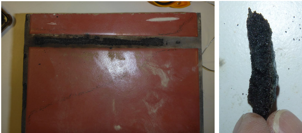
Figure 7.17: Charring of grout material
