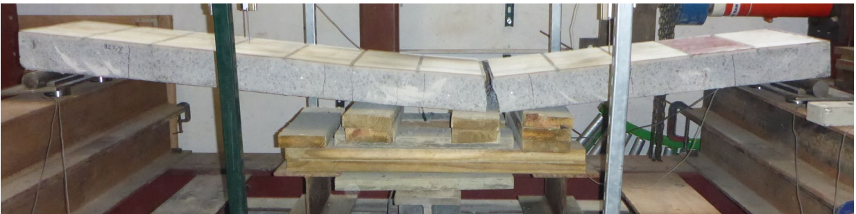
Figure 7.37: Photos of 300°C intact specimen load testing. Multiple flexural cracks in constant moment region during load application (top and middle); after failure (bottom)
