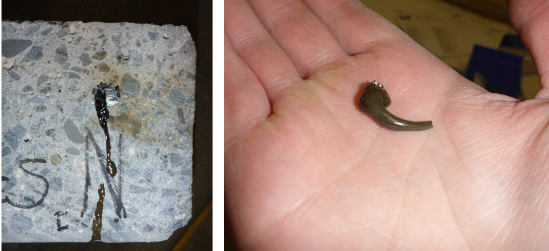
Figure 7.23: Melting of epoxy reinforcement coating
