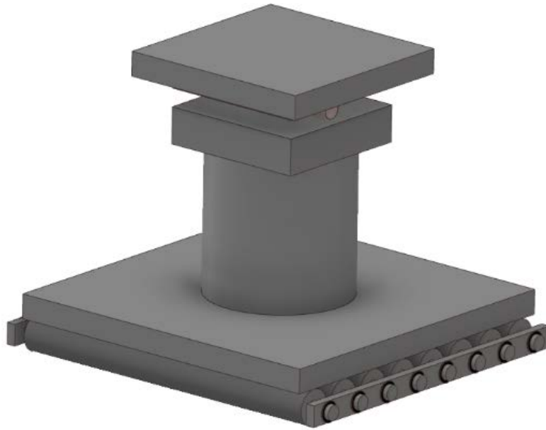
(a) Roller Support (1000 kip Load Cell)
