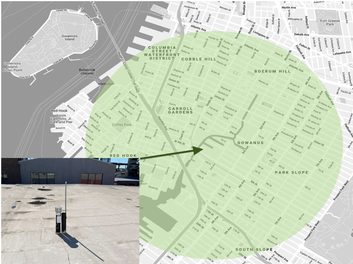
Figure 11: LoRaWAN gateway mounted (inset) with approximate 4km diameter coverage area highlighted in green
