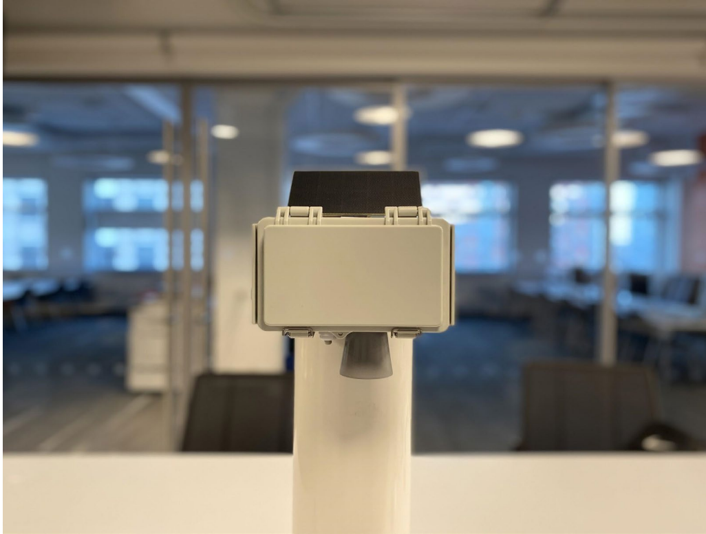
Figure 4: Prototype ultrasonic flood sensor mounted to a pole in sensors lab
