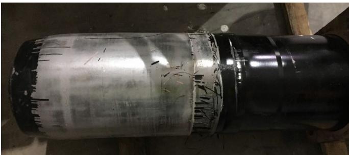
Figure 14. Deformed PBC deformation tube removed from the draft pocket
