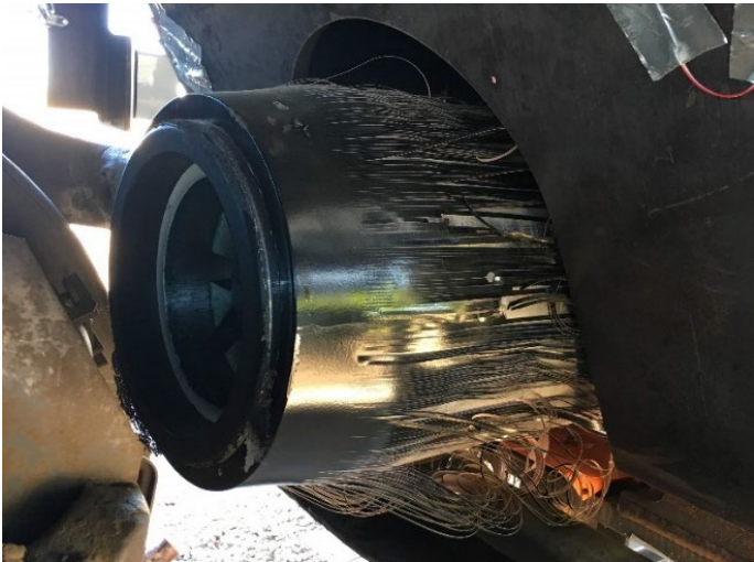
Figure 13. Post-test photograph showing the back of the deformation tube
