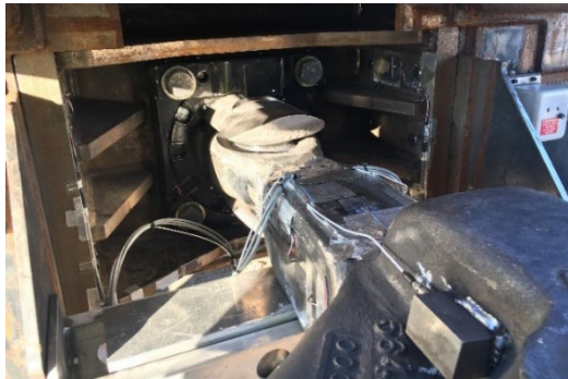
Figure 4. PBC installed within the sliding lug
