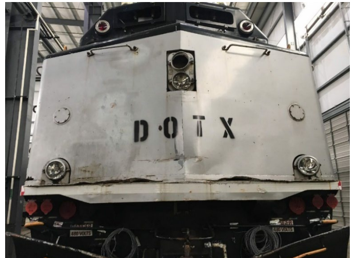
Figure 22. Conventional locomotive damage
