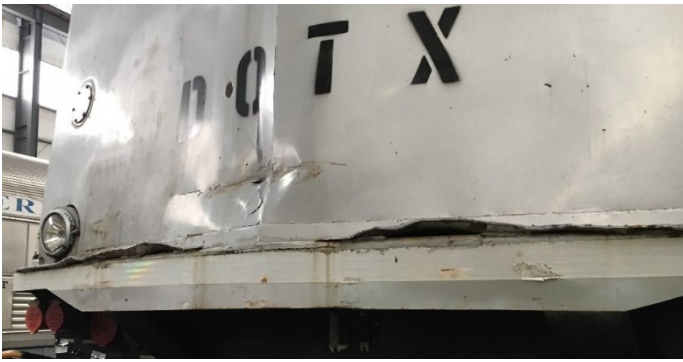
Figure 23. Close-up of conventional locomotive damage
