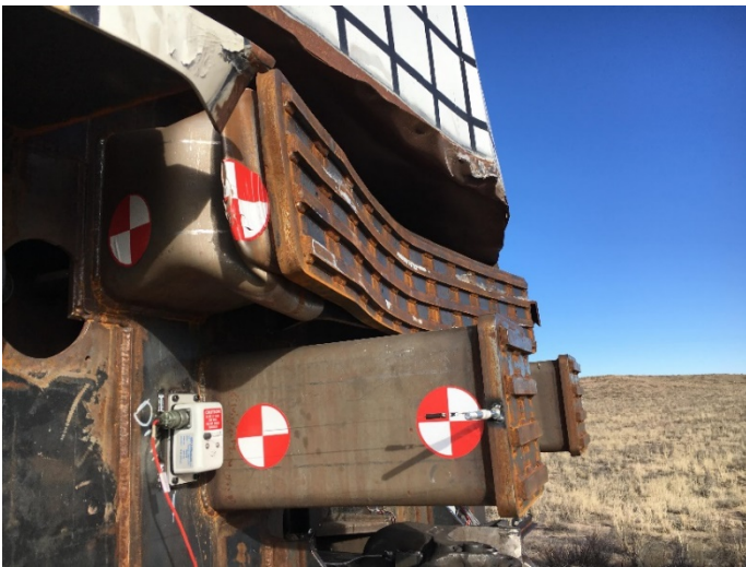
Figure 19. Post-test photograph of DAC showing that only the upper DAC tubes deformed
