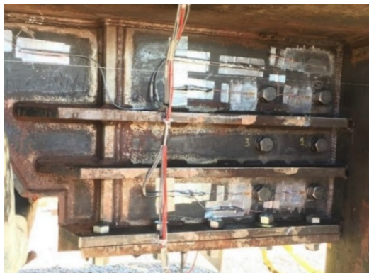
Figure 5. Exterior view of the shear bolts installed through the side plates of the draft pocket and into the side plates of the sliding lug
