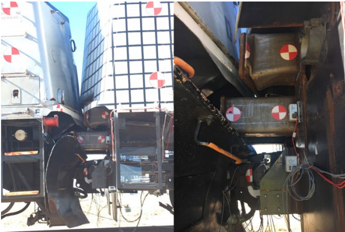
Figure 17. Post-test photo of CEM system; close-up on the right
