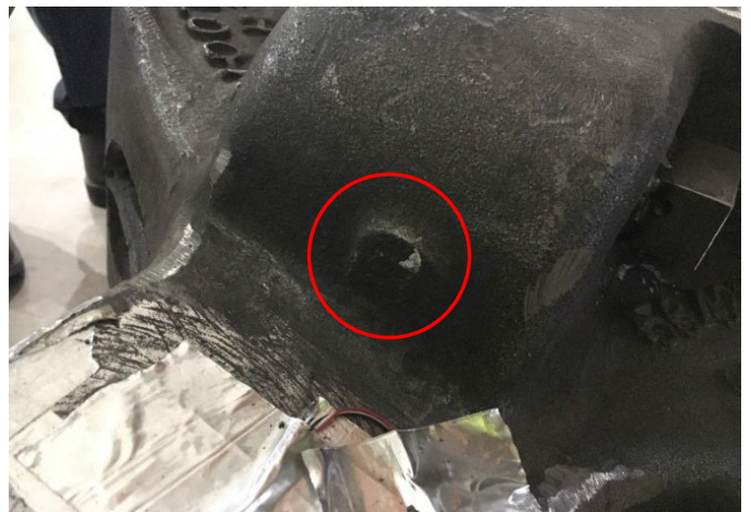
Figure 16. Damage to rear of the PBC coupler head from limit stop contact
