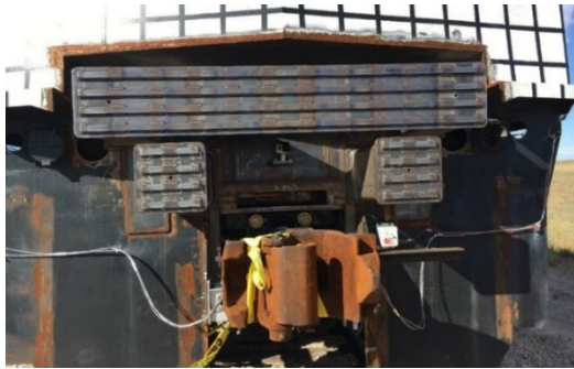
Figure 3. The DAC (top) and the PBC (bottom) comprise the locomotive CEM system
