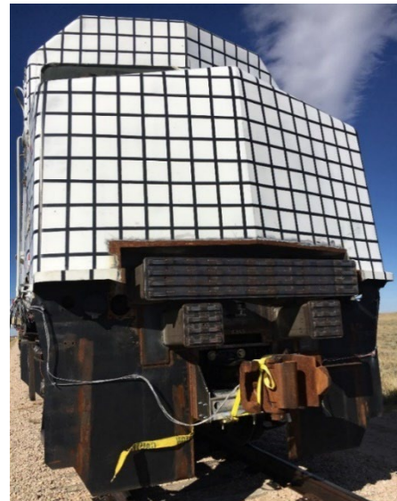
Figure 2. CEM Locomotive: F40 #234 retrofit with a PBC and DAC
