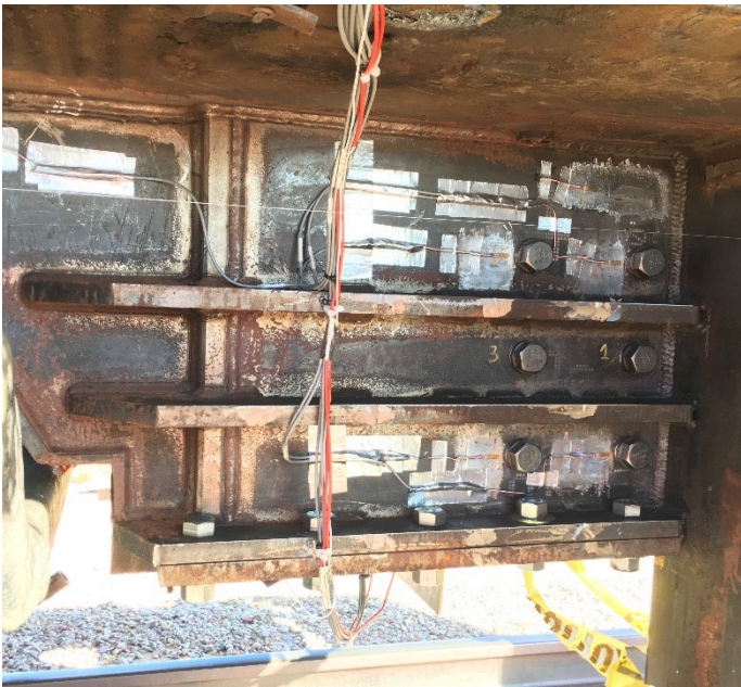
Figure 12. Strain gages on the CEM locomotive draft pocket exterior
