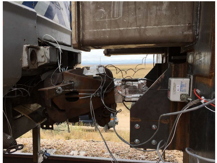
Figure 13. Photograph of longitudinal displacement transducer on PBC
