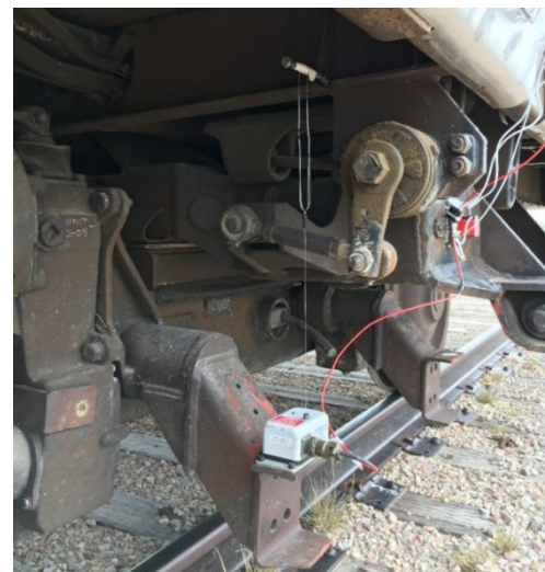
Figure 15. Photograph of vertical displacement transducer on CEM locomotive truck
