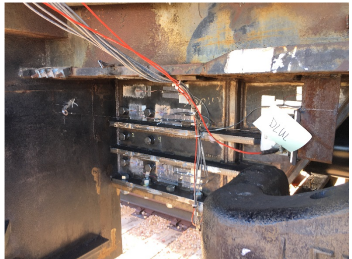
Figure 14. Photograph of longitudinal displacement transducer on CEM locomotive draft sill
