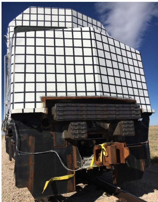
Figure 5. CEM Locomotive: F40 #234 retrofit with a PBC and DAC
