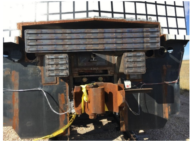
Figure 6. The DAC (top) and the PBC (bottom) comprise the locomotive CEM system
