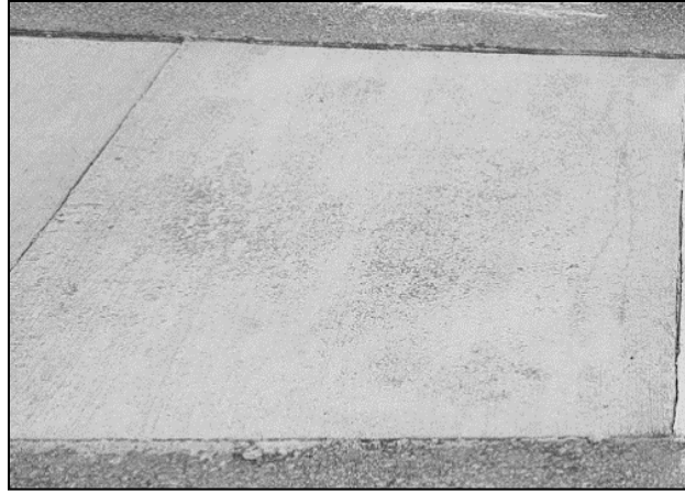
Figure 2.3: Panel B2 after application of \text{MgCl}_2 (December 18, 2019)
