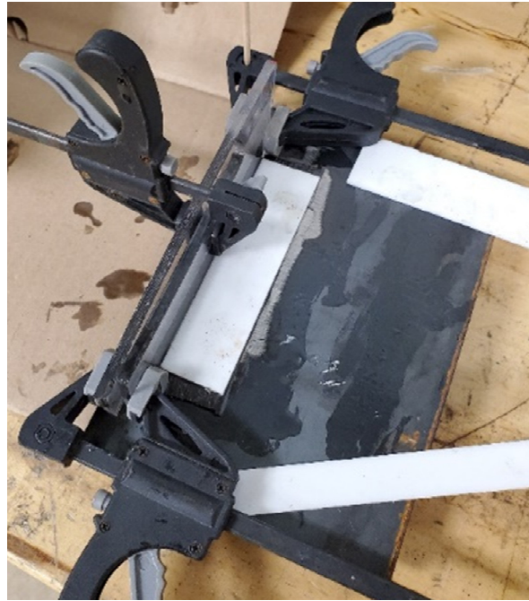
Figure 16. Layup method of CFRP showing clamps and acrylic molds
