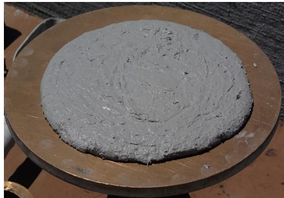
Figure 2-7 Fiber distribution in UHPC: (a) fiber uneven distributed during spread test (Photo credit: Torres); (b) fibers well distributed (Photo credit: Torres)
