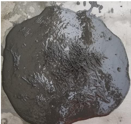
Figure 2-7 Fiber distribution in UHPC: (a) fiber uneven distributed during spread test (Photo credit: Torres); (b) fibers well distributed (Photo credit: Torres)
