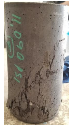
Figure 2-8 UHPC compressive strength: (a) experimental results (Singh et al. 2017), and (b) tested cylinder (Photo credit: Torres)
