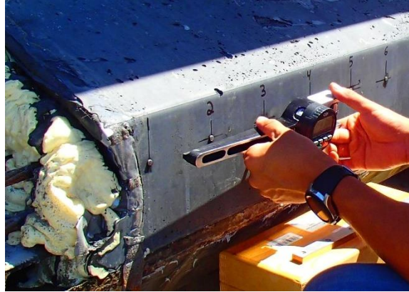
Figure 4-16 Transfer length measured using demec points and a digital length comparator
