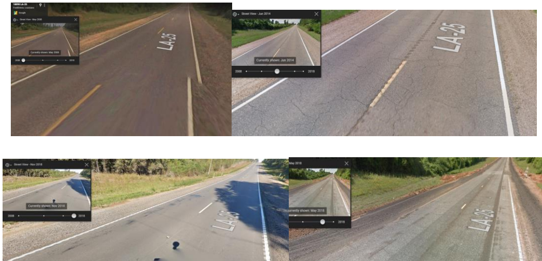
Figure B5. Change in Rumble Strips over the Years in Same Segment (Clockwise) – No Rumble Strips (May 2008), CLRS (June 2014), Construction (May 2018), SRS (November 2018)
