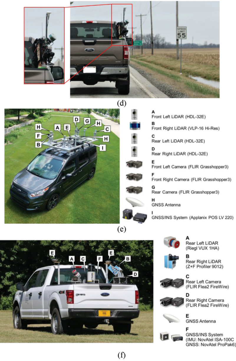
Figure 3.1 MLMS units used in this study: (a) unmanned aerial vehicle (UAV), (b) unmanned ground vehicle (UGV), (c) Backpack, (d) Mobile-pack, (e) medium-grade system (PWMMS-HA), and (f) high-grade system (PWMMS-UHA). All of these platforms are non-commercial systems designed and integrated by the research group.
