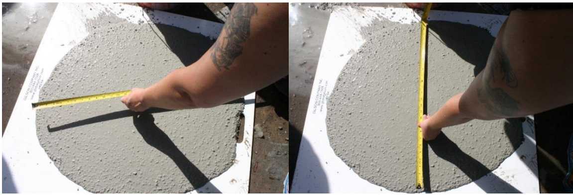
Figure 3.11 Measurement of spread for Argos SCC mix for shafts 47 to 52.
