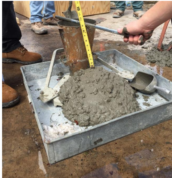
Figure 3.9 Measurement of 8.5-in. slump for shafts 19 to 22.
