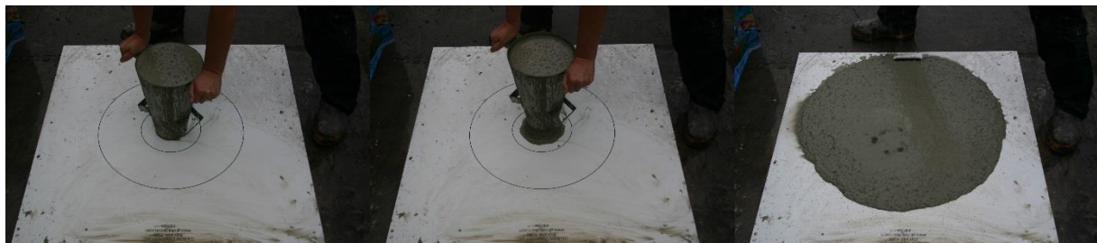
Figure 3.6 SCC slump/spread test where the standard slump cone is filled upside-down (left), the cone is lifted (center), and the diameter of the spread is measured (right).
