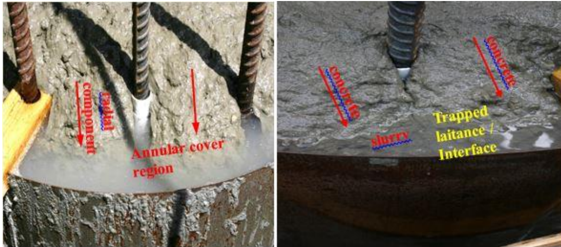
Figure 4.4.13 Experimental Study with Cast Shafts at USF, (Mullins, 2015): Flow Pattern Observed.
