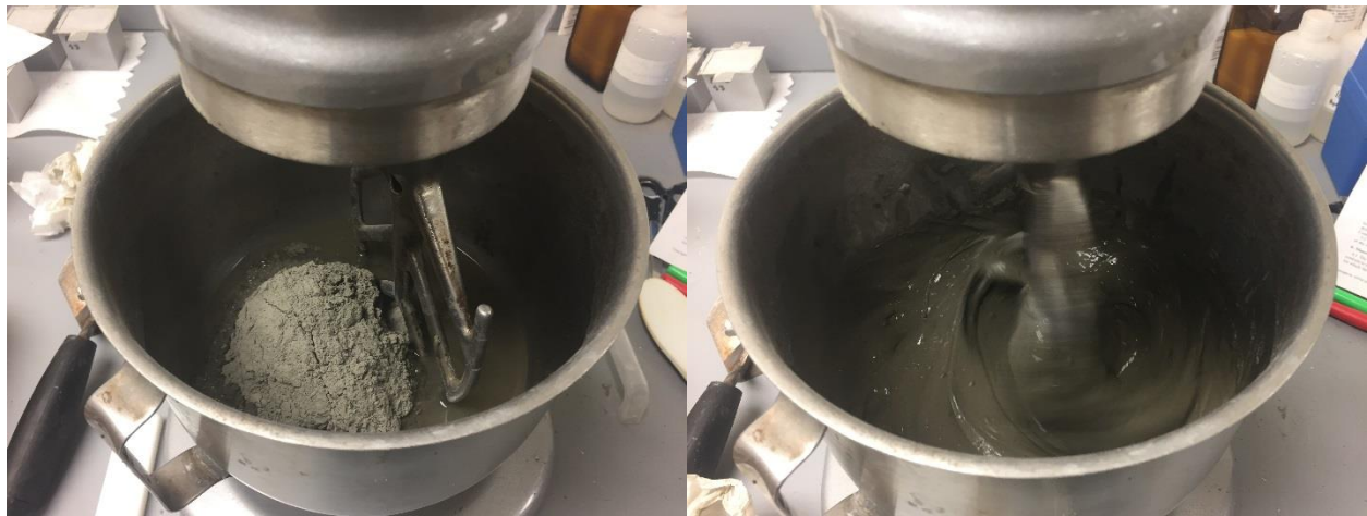
Figure 8.41 The addition of cement to water (left) and the mixing process (right).
