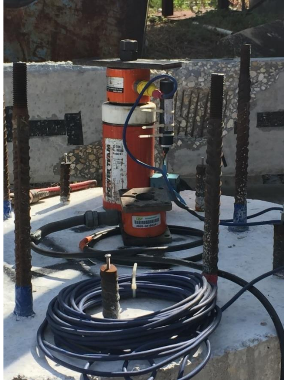
Figure 5.14 General assembly used for pullout testing: loading jack, load cell, steel plate, double nuts, and a displacement transducer.
