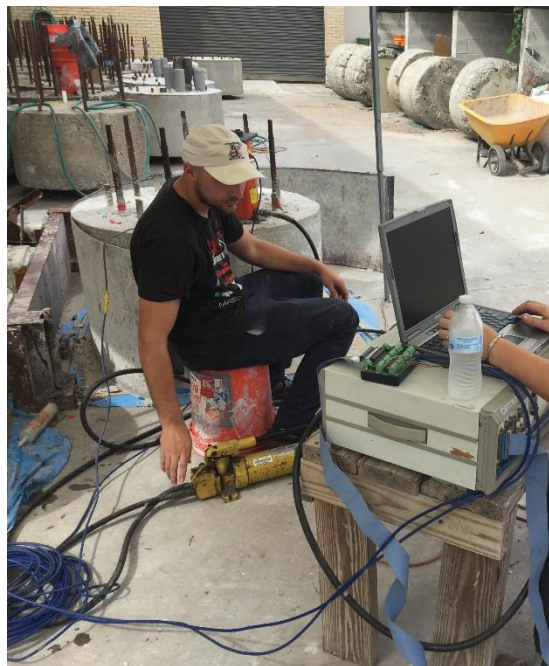
Figure 5.15 Testing of the pullout bars: as the bar is being loaded the computer is being monitored.
