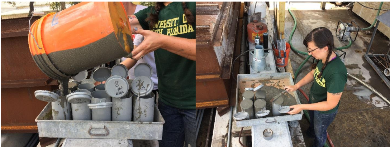
Figure 3.8 SCC cylinder preparation: pouring the concrete into cylinders (left) and leveling the tops (right).
