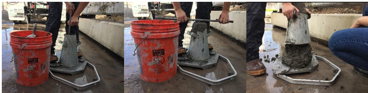
Figure 3.5 The phases of performing a standard slump test; from left to right: rodding 25 times per layer, leveling the top of the cone, removing the cone to measure the slump value.
