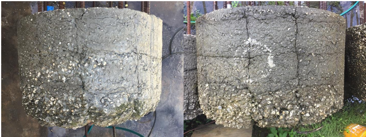
Figure 2.11 Shaft 4 55 sec/qt bentonite (left), shaft 5 90 sec/qt bentonite (right).
