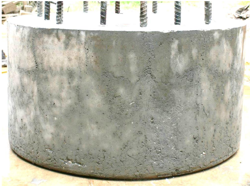
Figure 9.7 Shaft 11: f'_c 4530 psi; drilled shaft mix; 65 sec/qt polymer; smooth; no creases
