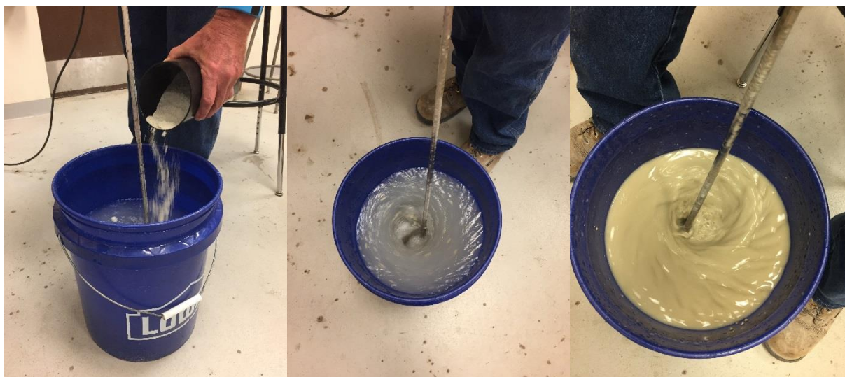
Figure 8.32 The bentonite powder slowly being added to the water (left) to form the slurry (middle and right).
