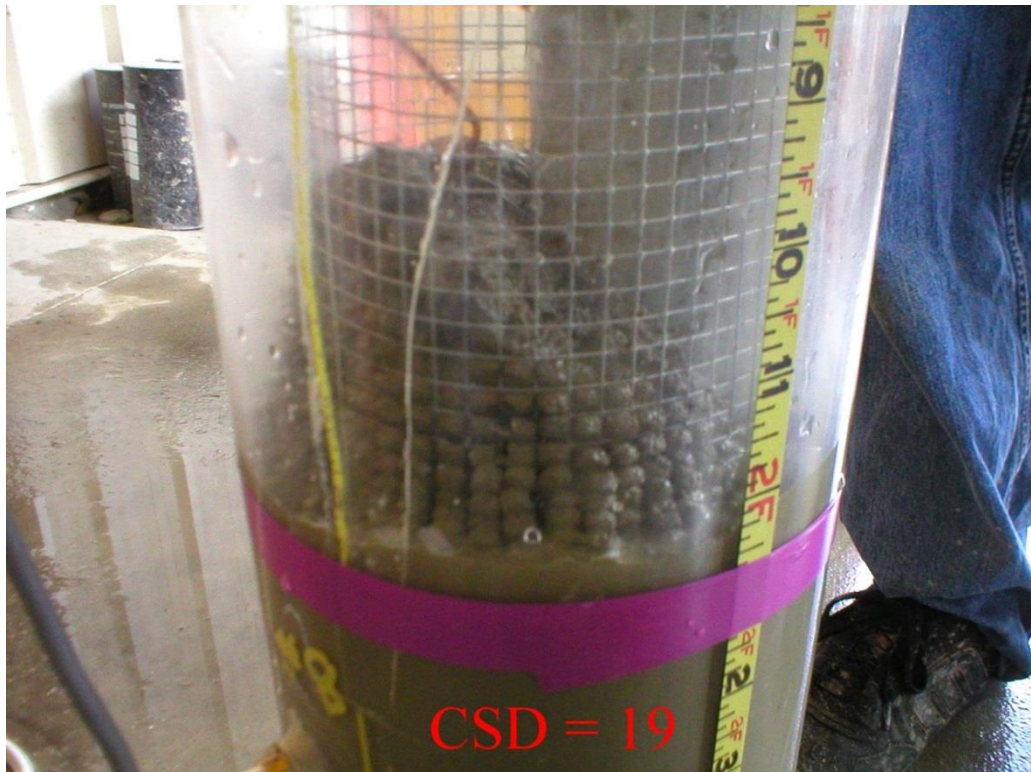
Figure 1.4 Laboratory tests with small-diameter aggregate and tight reinforcement (CSD = 19).
