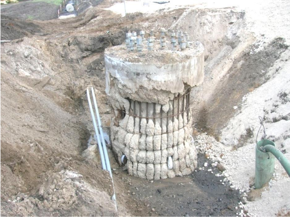
Figure 1.7 Shaft exhumed to show poor concrete flow performance from slurry properties or fresh concrete properties (courtesy of the FDOT State Materials Office).
