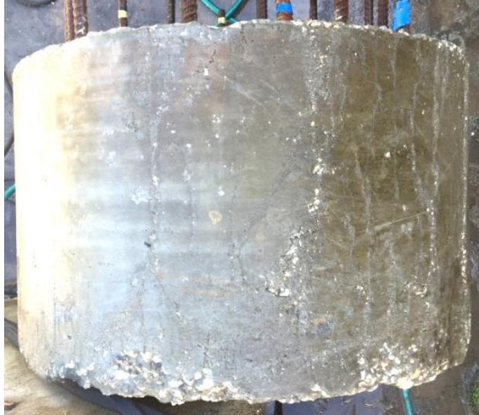
Figure 9.5 Shaft 6: f'_c 4358 psi; drilled shaft mix; water cast; smooth; faint channeling
