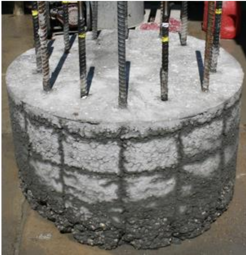
Figure 9.4 Visible mattressing after pressure washing
