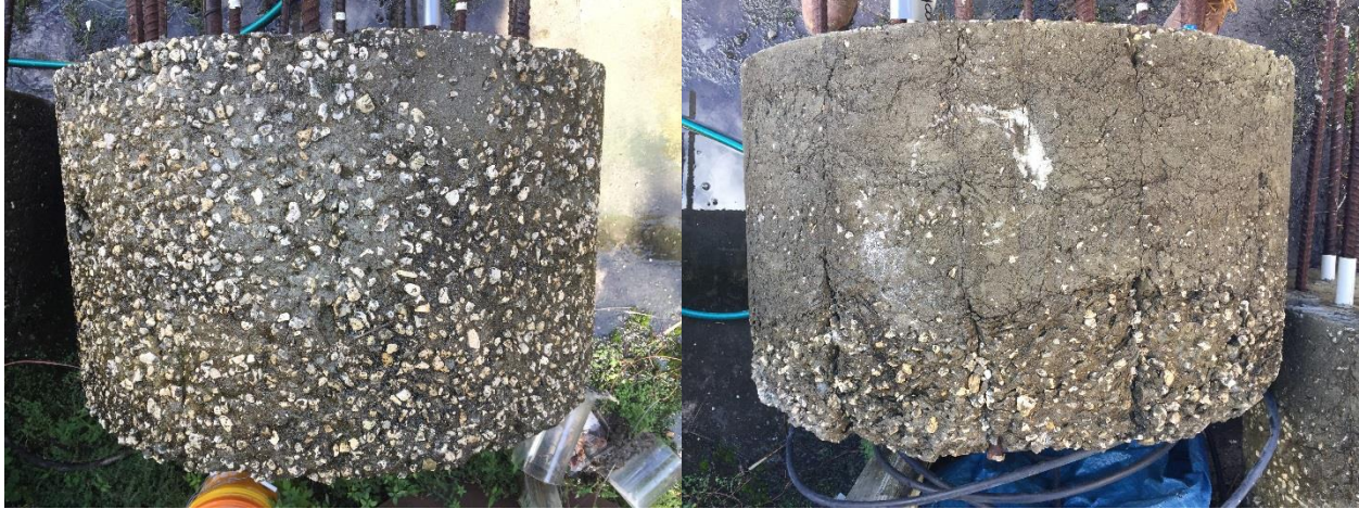
Figure 2.10 Shaft 7 30 sec/qt bentonite (left), shaft 8 40 sec/qt bentonite (right).
