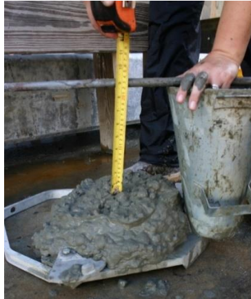
Figure 3.12 Measurement of 9-in. slump for shafts 53 to 58.
