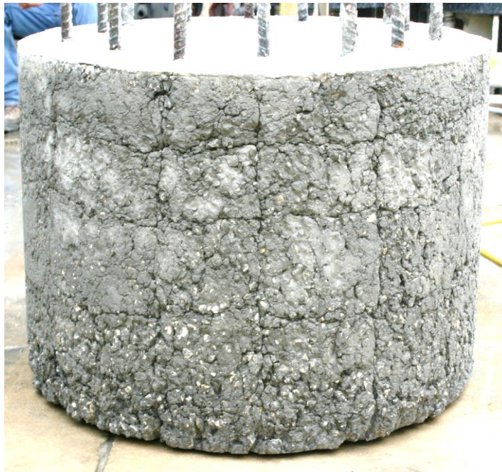
Figure 9.6 Shaft 9: f'_c 4530 psi; drilled shaft mix; 50 sec/qt bentonite; rough; with well-defined creases
