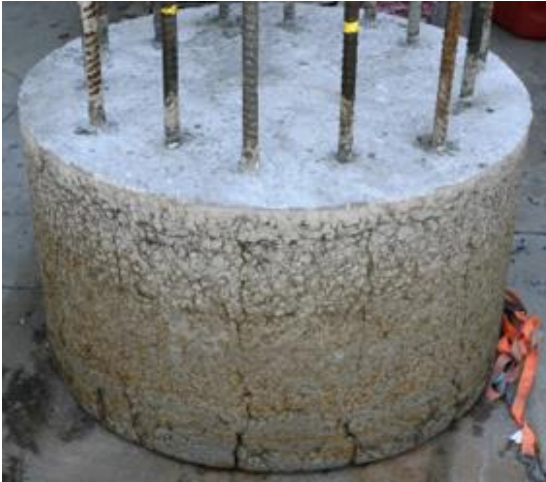
Figure 9.2 Visible mattressing upon form removal.
