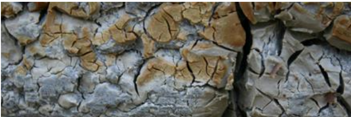
Figure 9.3 Bentonite caked to the concrete surface trapped between concrete and casing.
