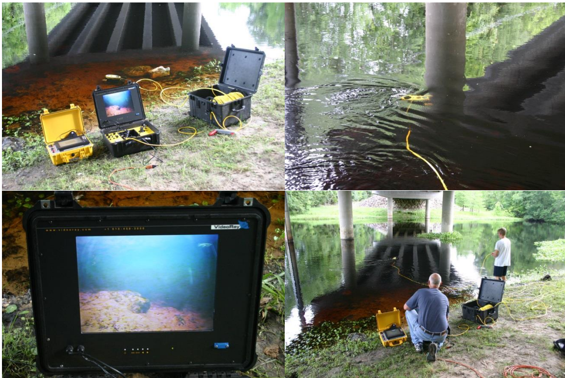
Figure 10.53 Remote operated vehicle system used to capture underwater images without divers.
