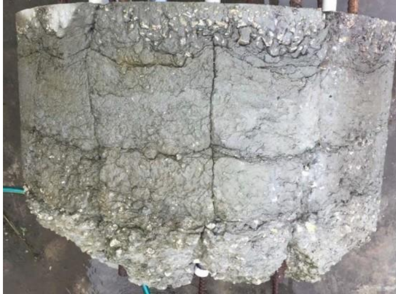
Figure 2.8 Mattressing on a drilled shaft test specimen.
