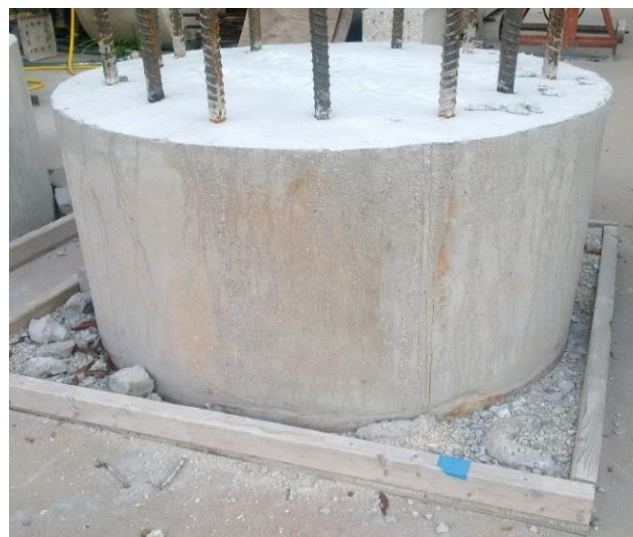
Figure 4.4.39 Experimental Study with Cast Shafts at USF, (Mullins, 2015): Flow Performance of SCC Shaft Cast under Water- Shaft Size 48-inch Diameter.
