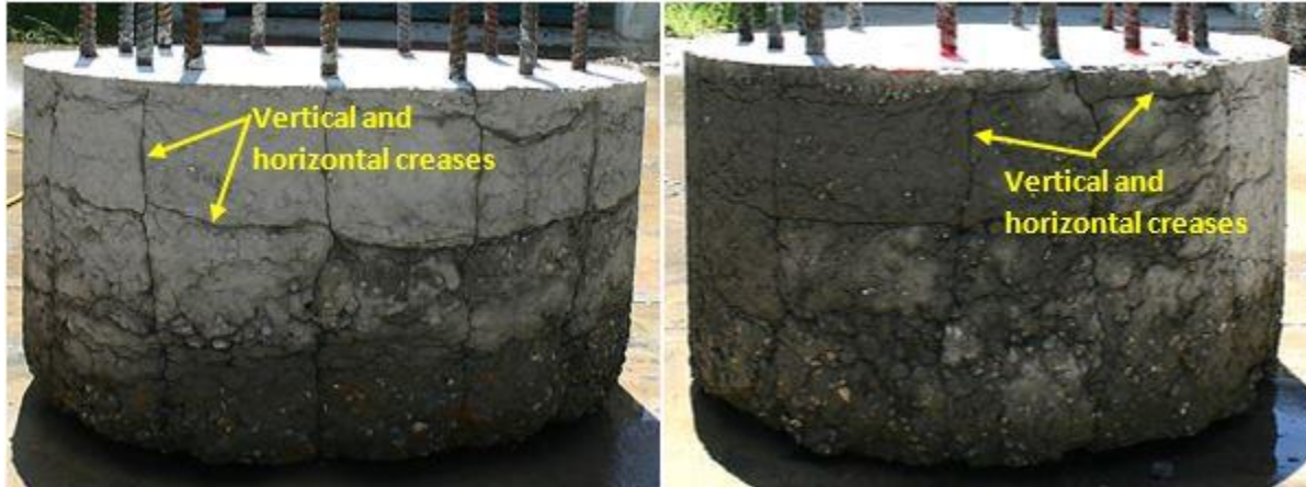
Figure 4.4.21 Experimental Study with Cast Shafts at USF: Vertical and Horizontal Creases Observed at the Edge of Cast Shaft, (Mullins, 2015).
