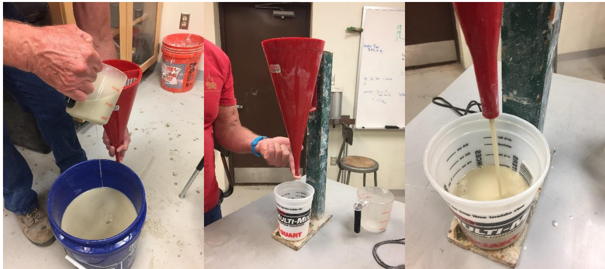
Figure 8.33 Testing of the bentonite slurry viscosity using the Marsh funnel.
