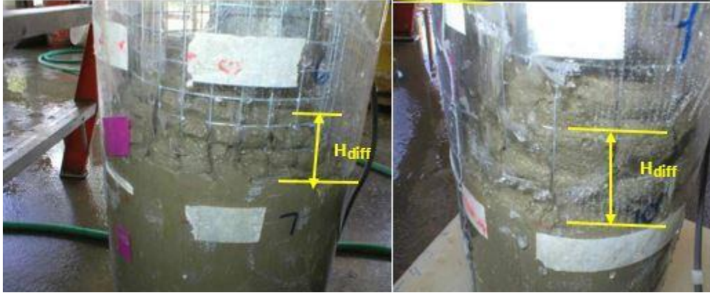
Figure 4.4.23 Laboratory LCP Test at USF: Flow Pattern of Rising Mortar with Head Differential, (Mullins and Ashmawy, 2005).
