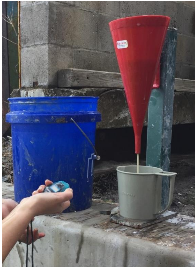
Figure 2.6 A Marsh funnel viscosity test in progress.
