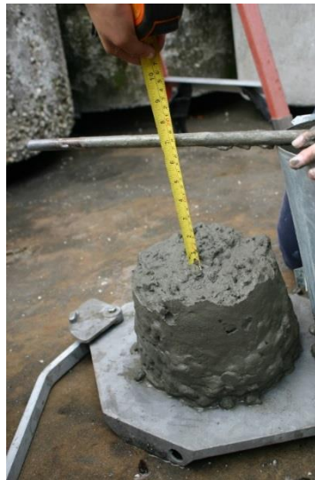
Figure 3.10 Measurement of 7-in. slump for shafts 31 to 36.
