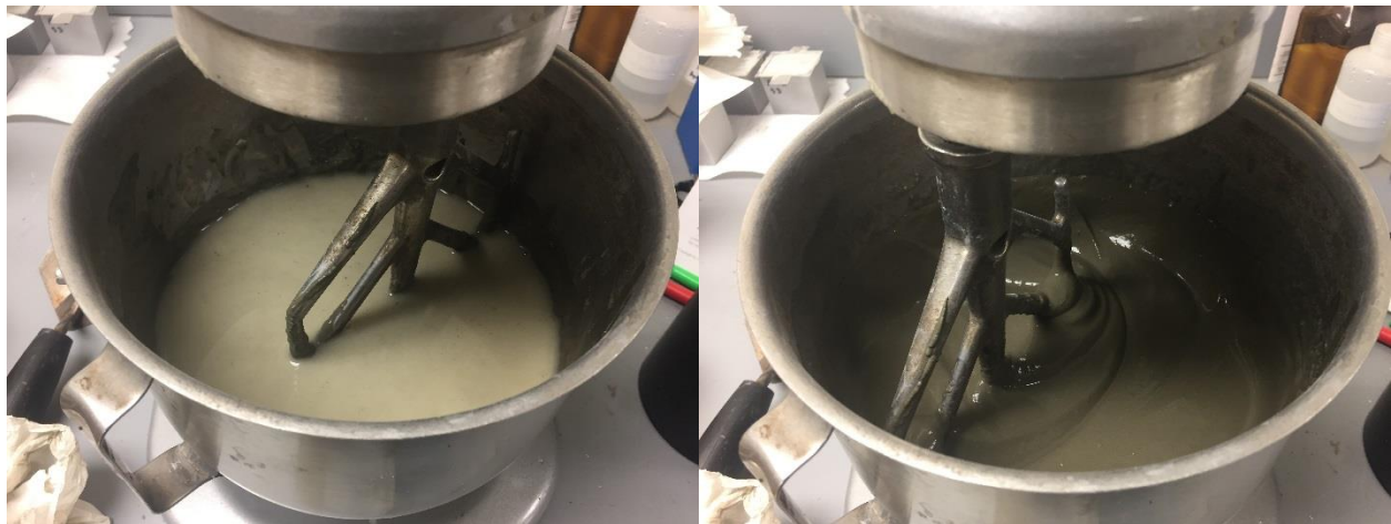
Figure 8.42 The addition of bentonite slurry to the mix (left) and the mixing process (right).
