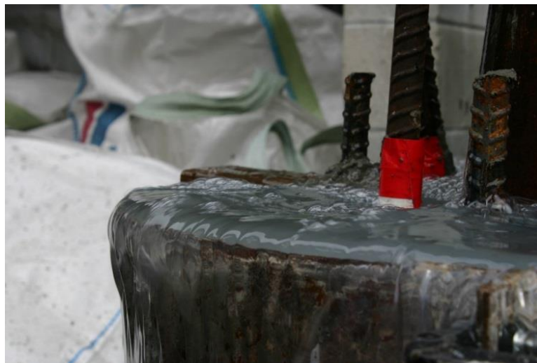
Figure 2.5 Close-up of a thicker viscosity polymer slurry exiting the form.
