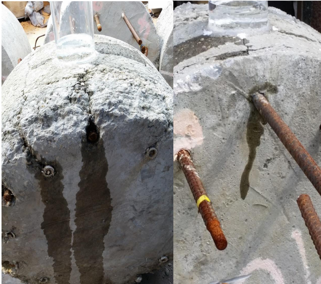
Figure 6.3 Water leaking below reinforcement in the bottom (left) and the top (right) of the shaft
