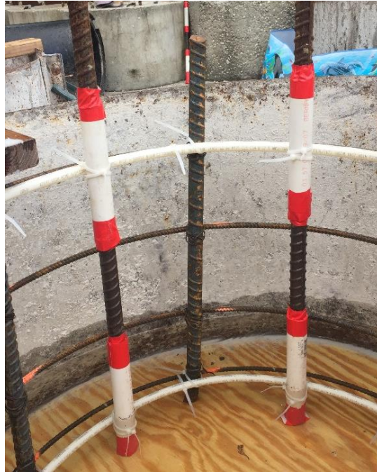
Figure 3.4 The six -six-inch debonded section of bar through the use of PVC pipe sections.
