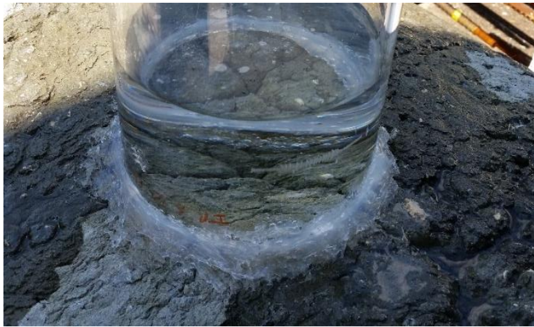
Figure 6.1 Water filled tank attached to concrete surface
