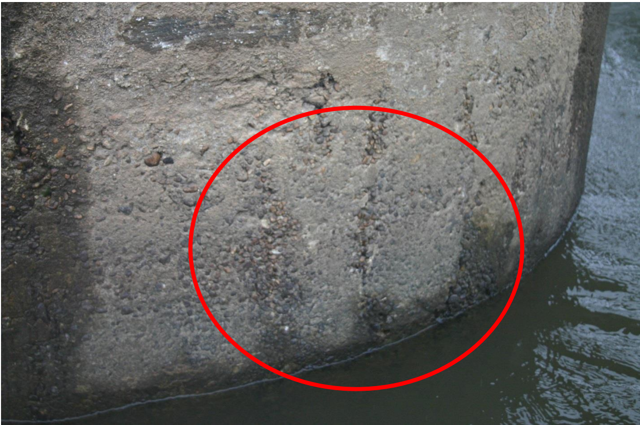
Figure 10.65 West side of test shaft 8, light creases from vertical reinforcement.
