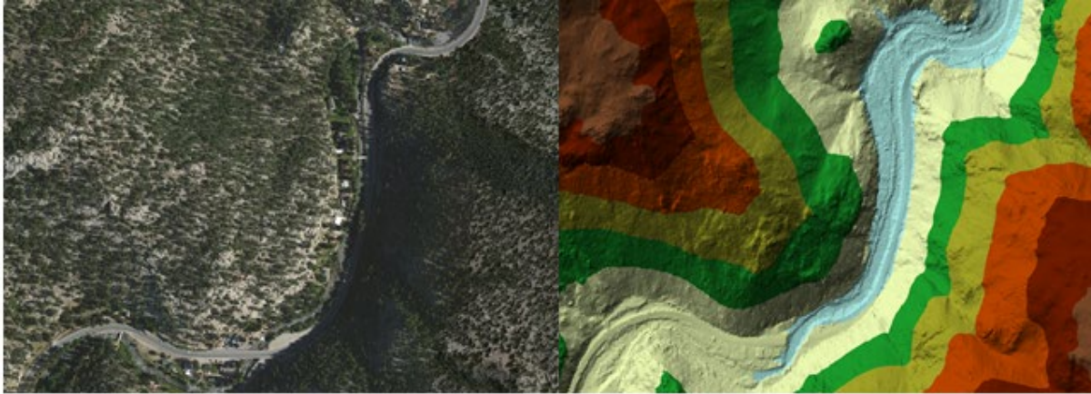
Figure 1.2 Topography the Big Thompson Canyon with elevations ranging from 8100-7150 feet located slightly downstream from Estes Park at bridge C-15-AM. This was generated via ArcMap in combination with LiDAR data provided by Colorado GeoData.
