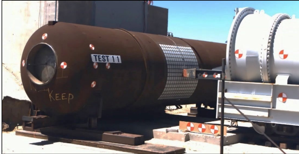
Figure 9. Ram Arm with 12-inch by 12-inch Indenter Aligned with Impact Zone on the Tank Car
