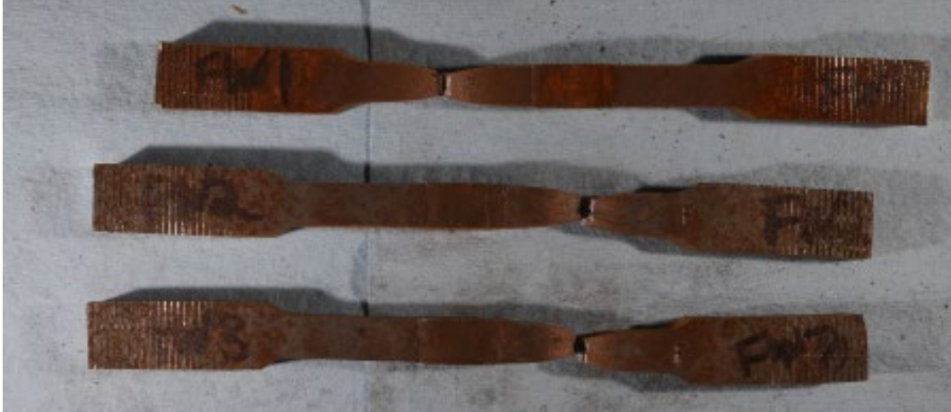
Figure B57. Post-test Factory Weld ASTM-E8 Tensile Coupons
