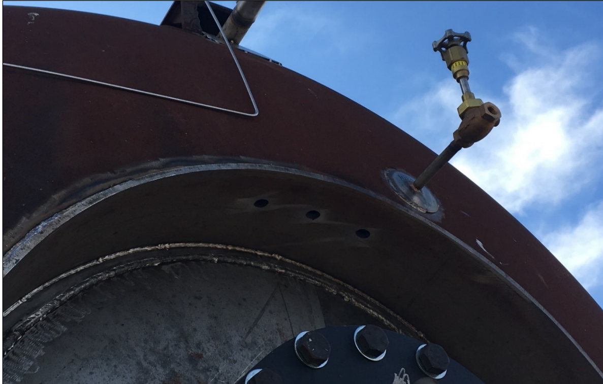
Figure 6. Pipe Used for Setting Innage and Pressurizing the Tank Car
