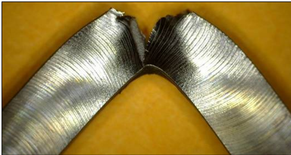
Figure B97. View of Exemplar Post-test CVN Coupon Fracture Surface
