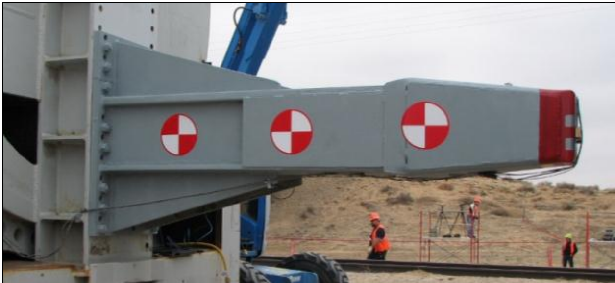
Figure 8. Ram Arm with 12-inch by 12-inch Indenter
