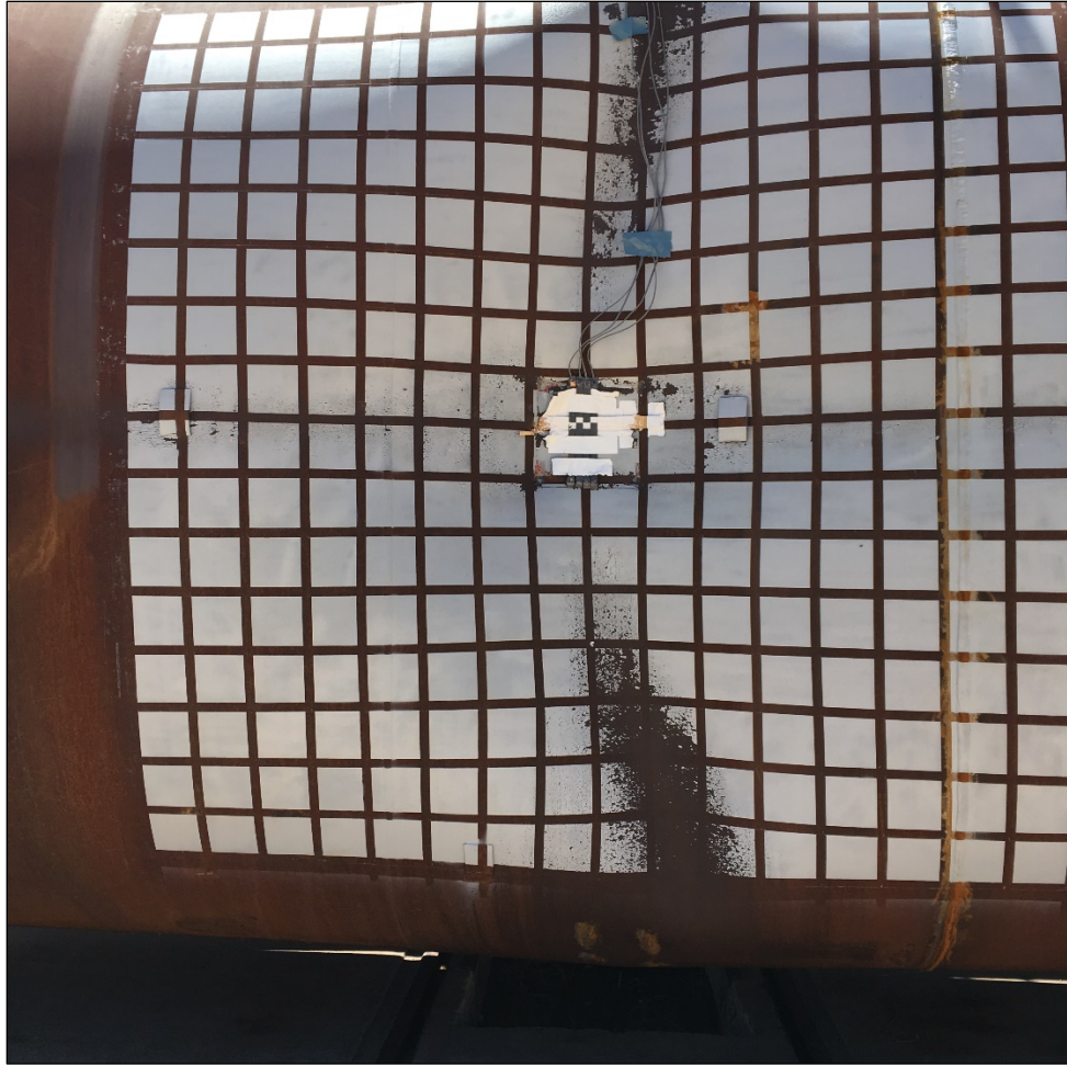
Figure 19. Tank Car After the Impact (impact side)
