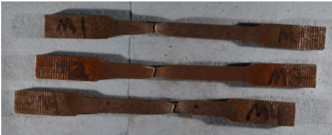
Figure B56. Post-test Parent Material ASTM-E8 Tensile Coupons
