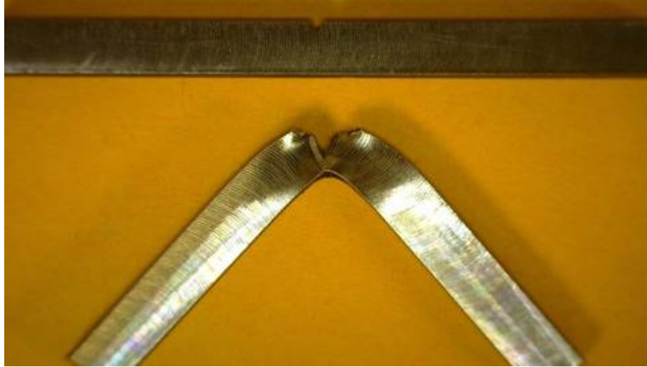
Figure 37. Pre- (top) and Post-test (bottom) CVN Specimens
