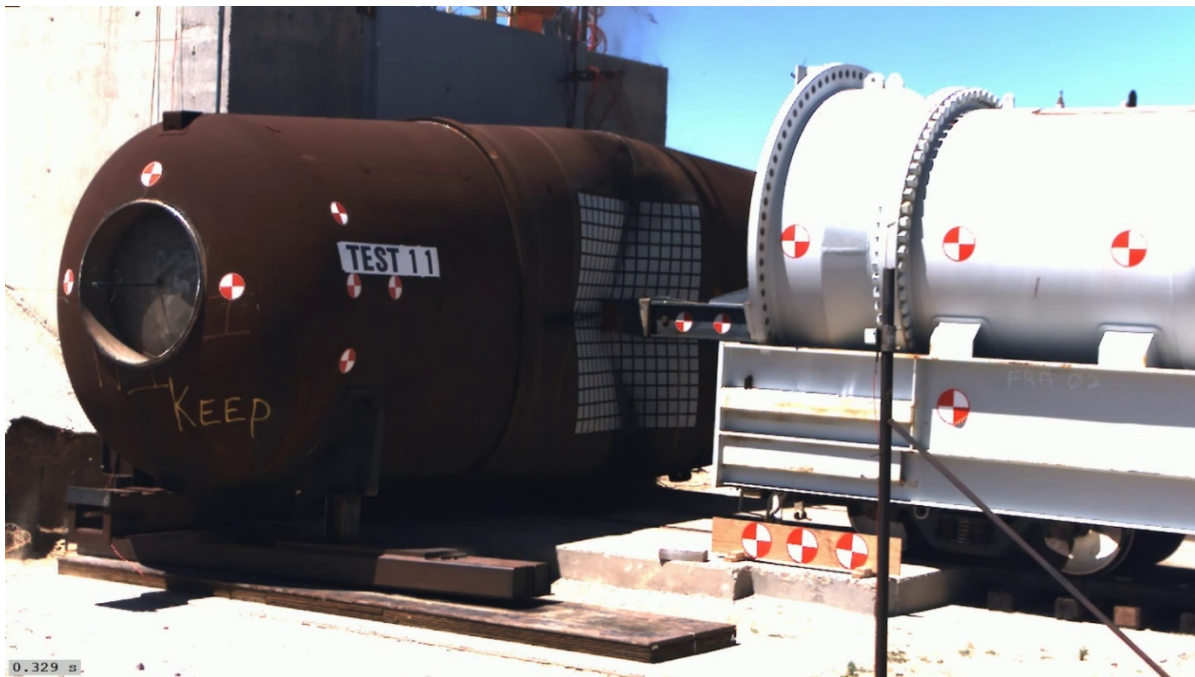
Figure 23. Still Frame from High-speed Video Taken at Approximate Time of Maximum Indentation (0.329 seconds)
