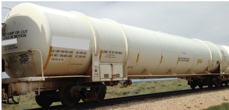
Figure G1. DOT-113 Tank Car Used in Test 10
