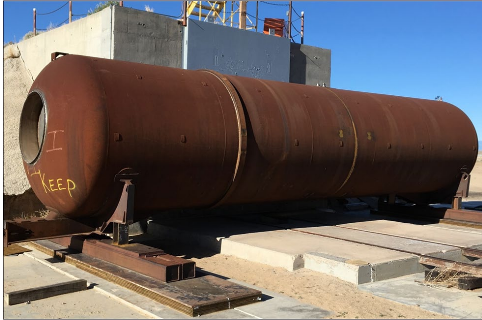
Figure 2. DOT-113 Surrogate Tank Car Mounted on Support Skids
