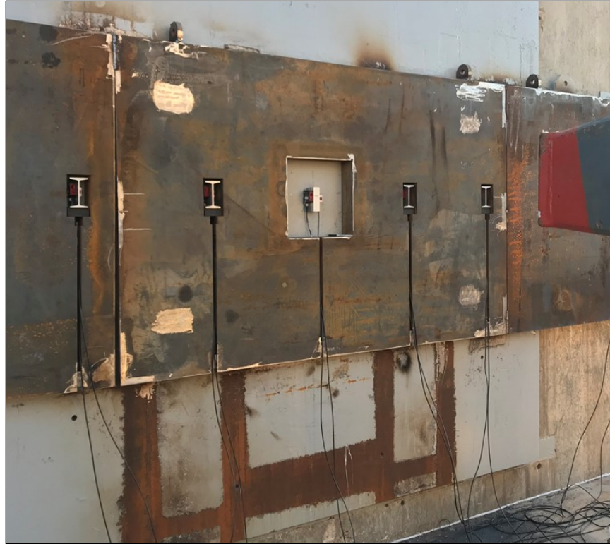
Figure 17. Lasers Displacement Transducers on Crash Wall
