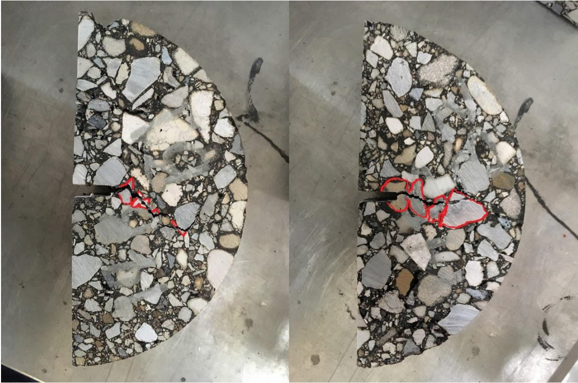
Figure 5.14 Comparison of Crack Propagation between Specimen 14-B-B1 (Left, Slope = -1.43 kN/mm, FI = 6.4) and 14-B-B2 (Right, Slope = -2.82 kN/mm, FI = 3.0).
