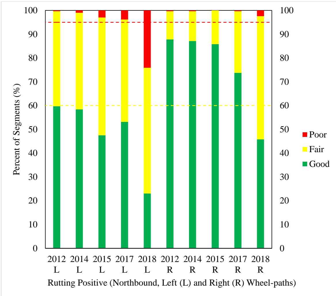
Figure 3.8 Comparison of Right and Left Wheel-Path Rutting for the Positive Direction
