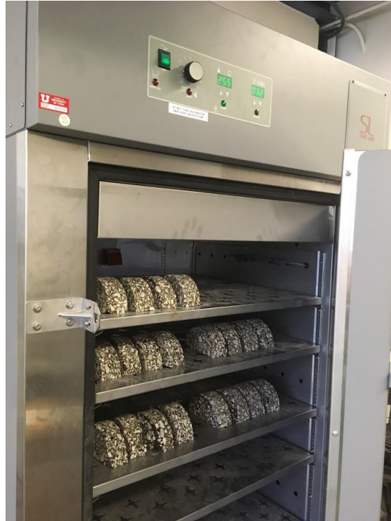
Figure 5.12 Half-Disc Specimens Curing in the Environmental Chamber
