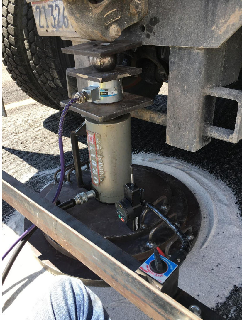
Figure 2.2 Plate Load Test Setup
