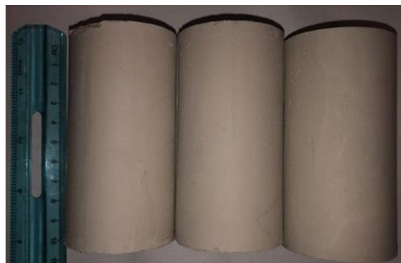
Figure 4-4-1 Laboratory prepared cylindrical specimen of synthetic mudstone for UCT and triaxial testing.
