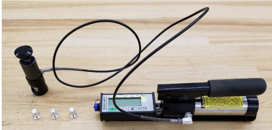
Figure 3. Pull Off Tester and 20 millimeter Pull Off Dollies
