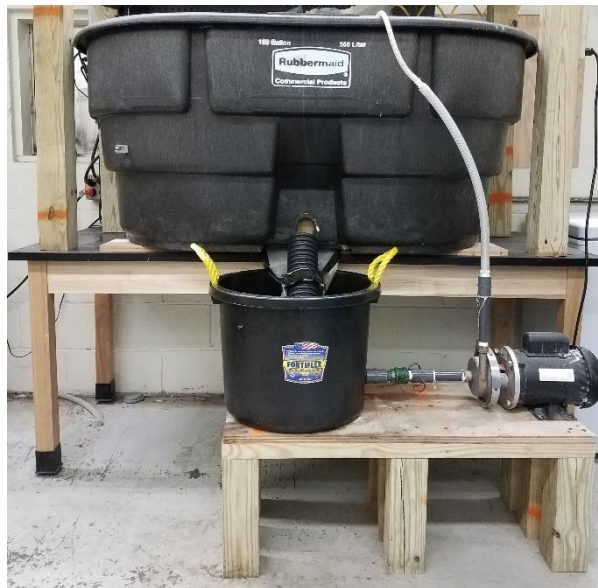
Figure A1. Polyethylene Plastic Tub with a Capacity of 150 Gallon and Salt Water Solution Reservoir
