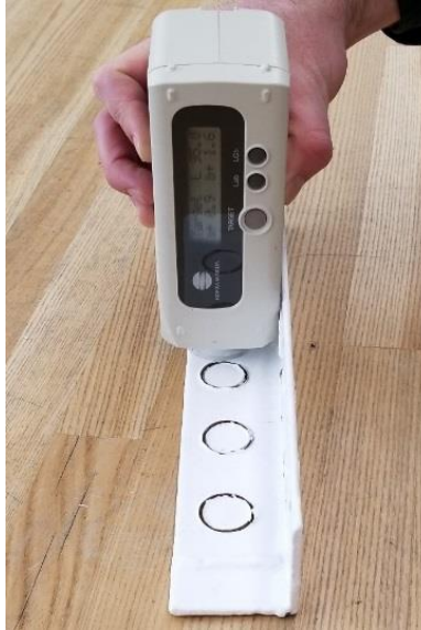
Figure 5. Konica Minolta CR-10 Plus Color Reader
