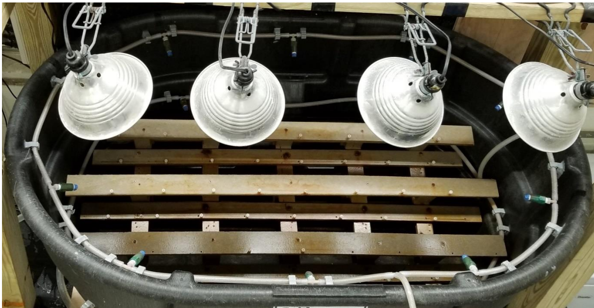
Figure A3. Salt Sprayer Layout
