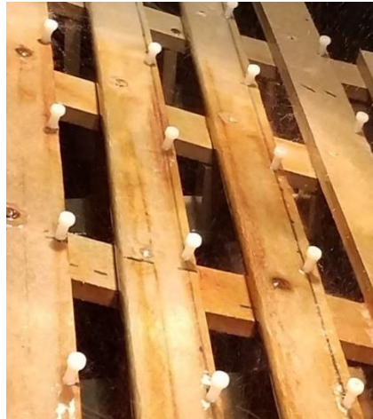
Figure A7. Shoulder Screws Installed on the Specimen Holding Rack to Prevent Slipping
