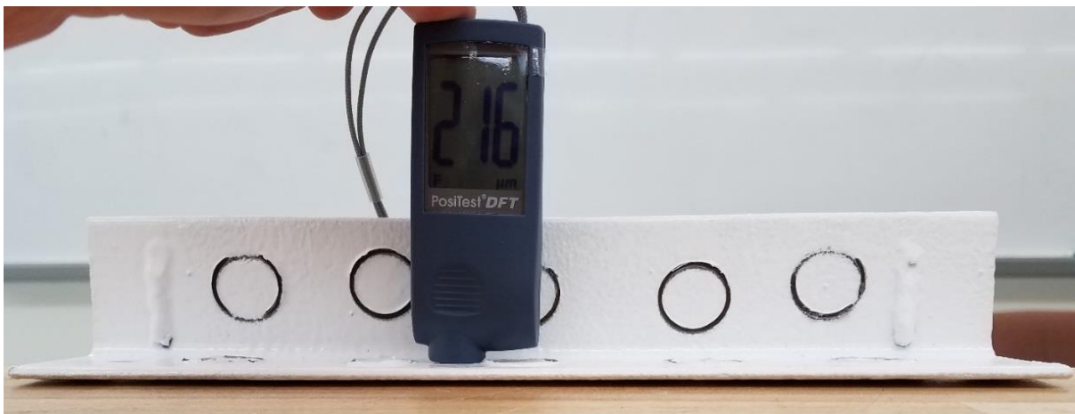
Figure 4. Thickness gage used for measuring the thickness of paint layers
