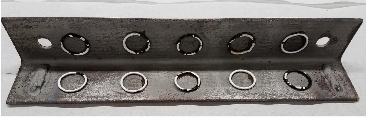
Figure 10. O-rings attached to steel specimen
