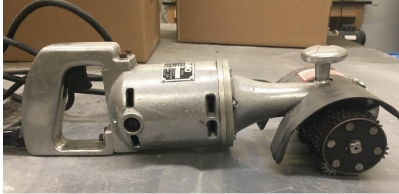
Figure 6. Aurand hand-held steel toothed cleaning machine
