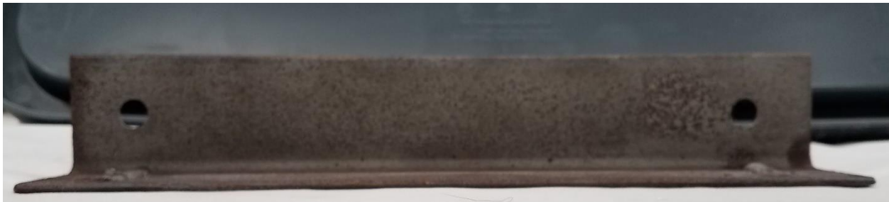
Figure B1. Typical ½ inch diameter holes in steel specimens
