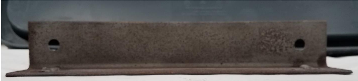
Figure 8. Typical ½ inch diameter holes in steel specimens
