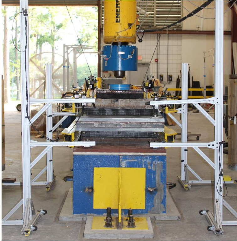
Figure B-18 Supporting frames for DX laser gauges
