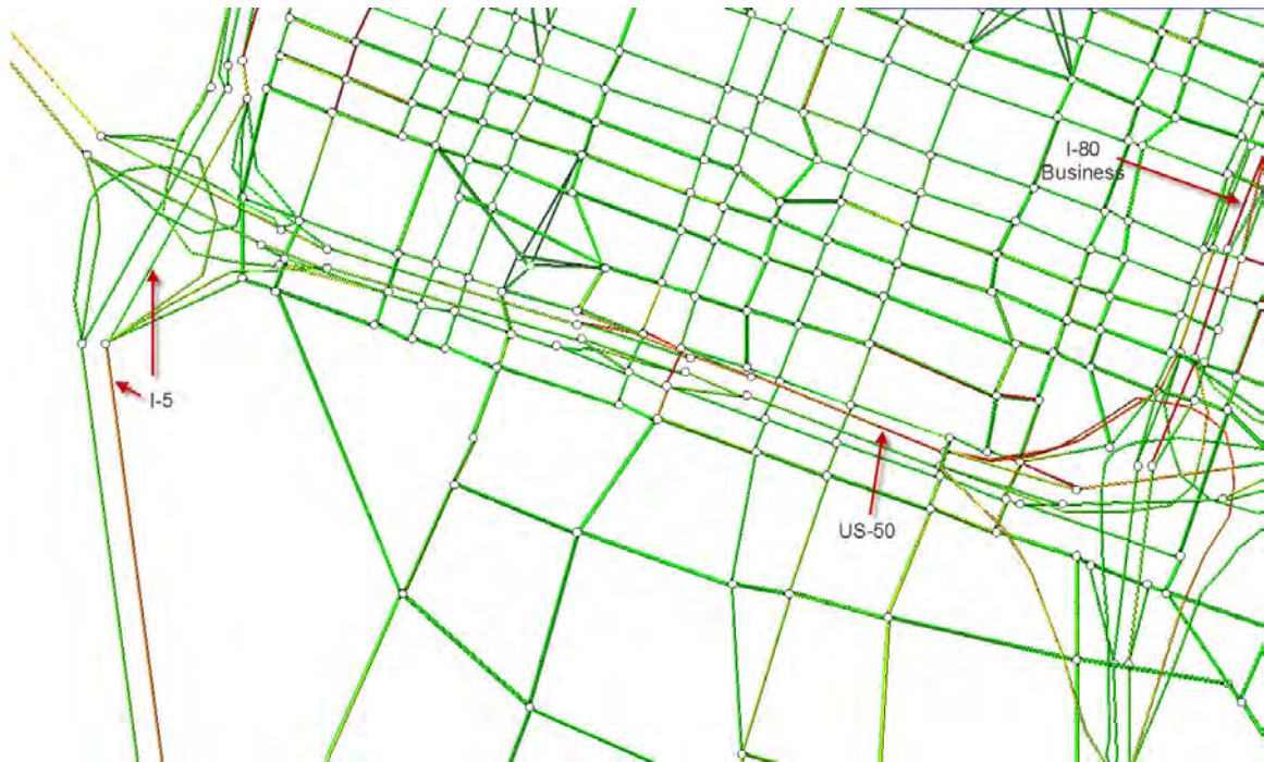
Figure 4.9: A snapshot of the queues on I-80 and US-50 at 8:00am during the directional NB closure in the actual plan (morning peak)
