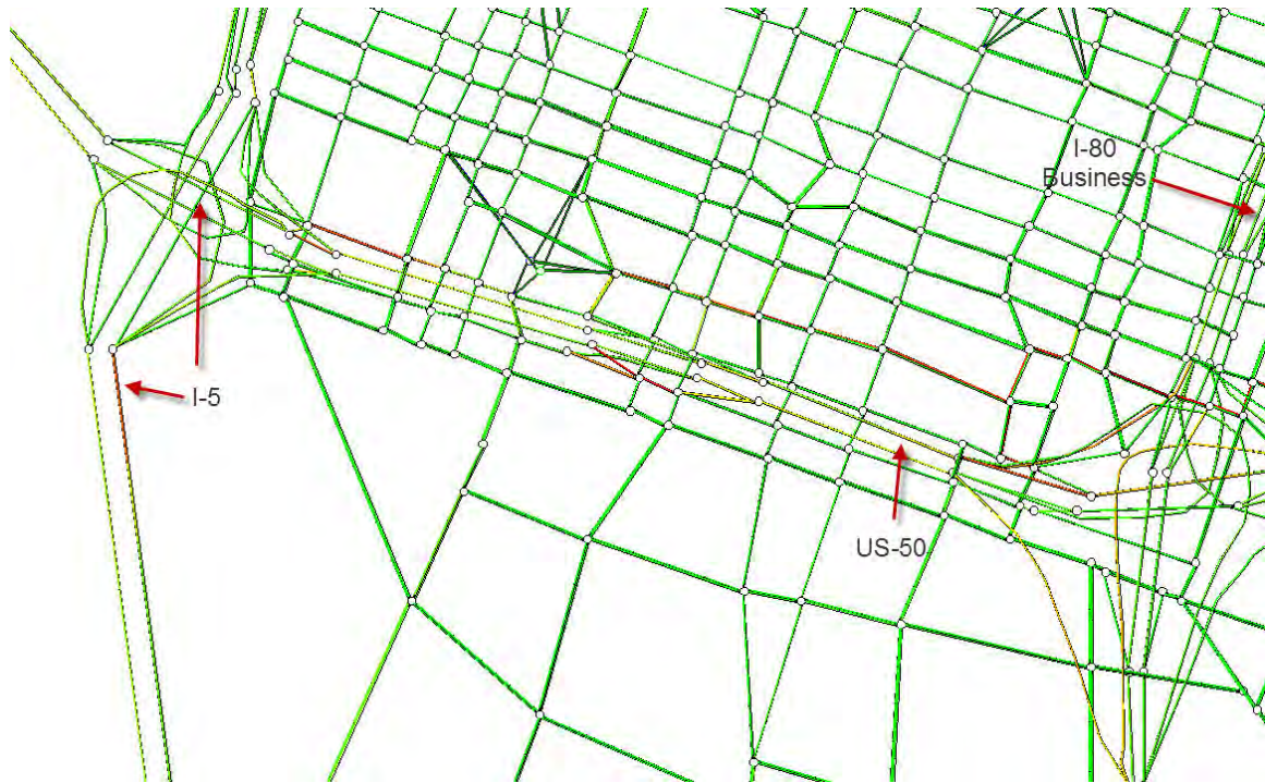
Figure 4.8: A snapshot of the queues on I-80 and US-50 at 8:00am for the baseline (morning peak)
