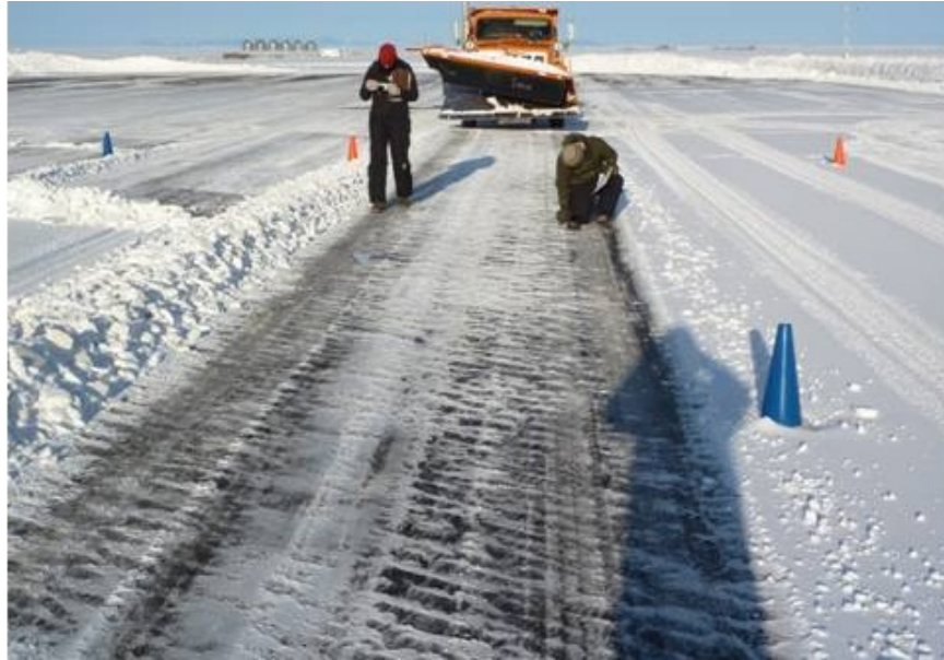
Figure 43: A typical test section after plowing.
