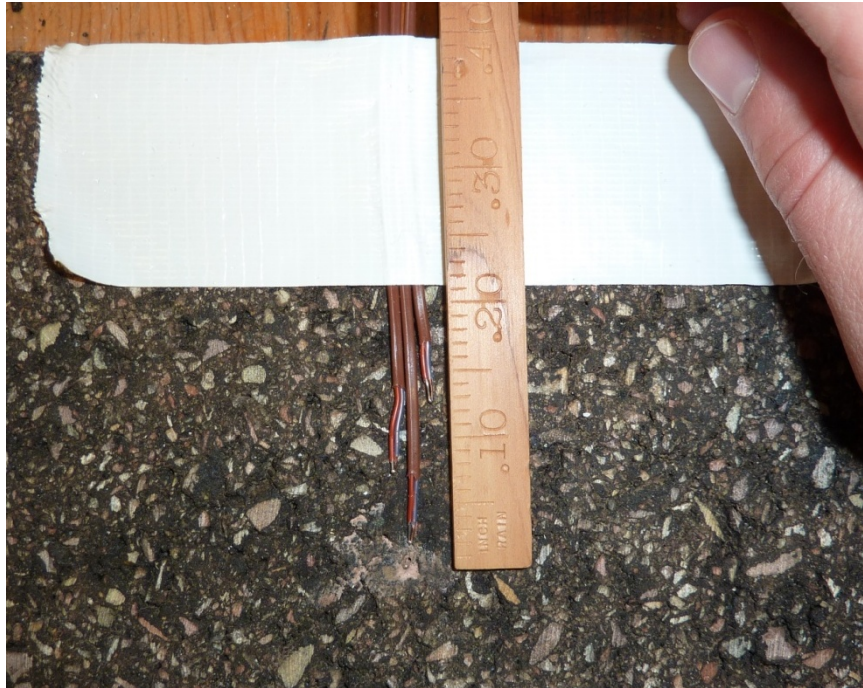
Figure 22: Positioning of thermocouples under the snow sample.
