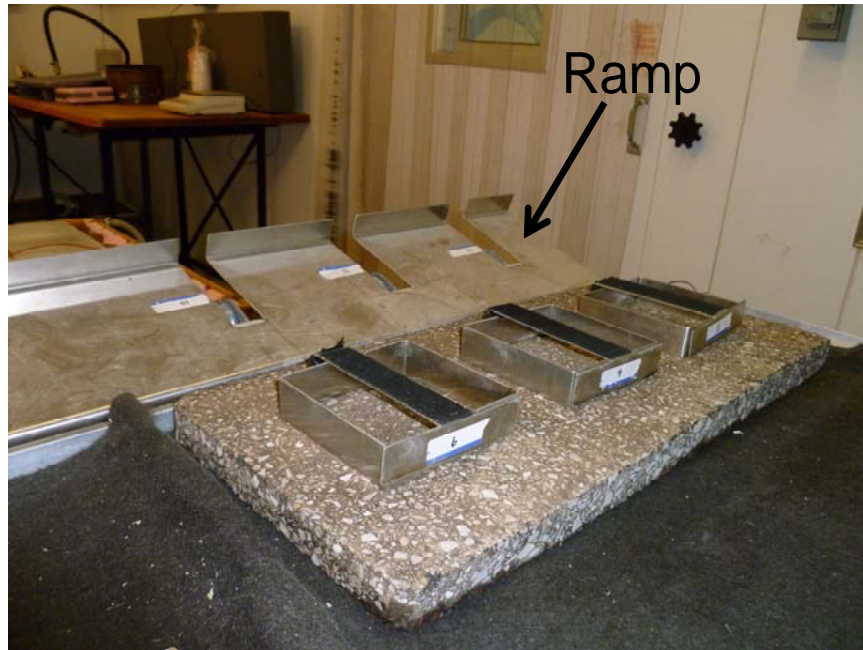
Figure 14: Ramps on the temperature-controlled table.
