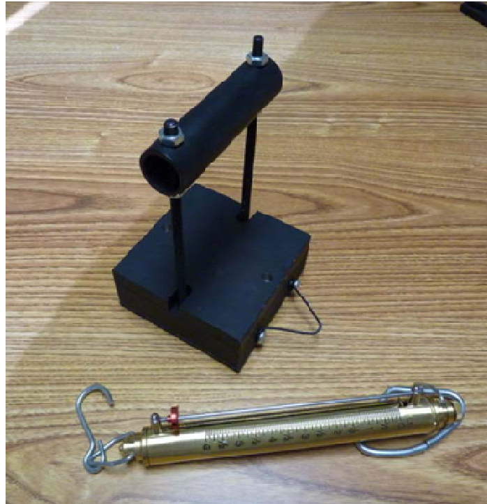
Figure 15: Friction tester and spring scale.
