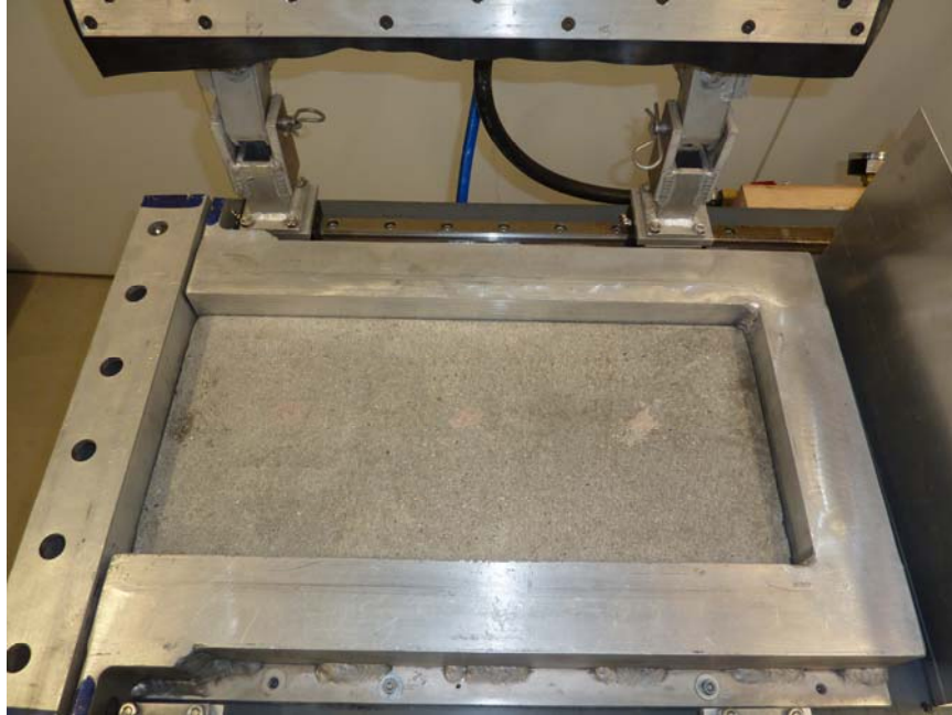
Figure 6: Pavement sample in the compaction box.
