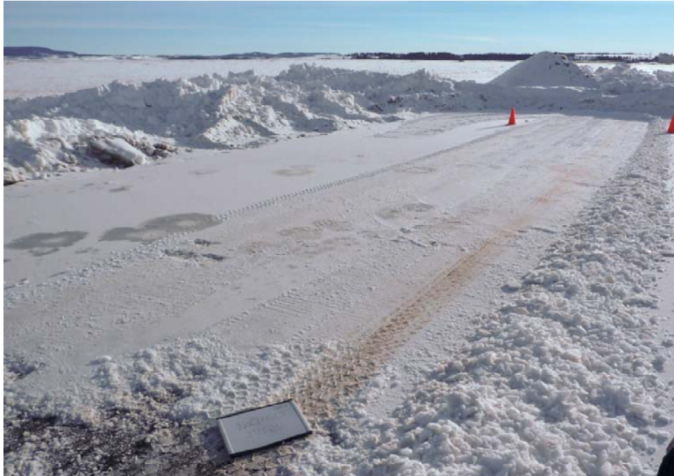
Figure 42: Icy test sections after two attempts at plowing.
