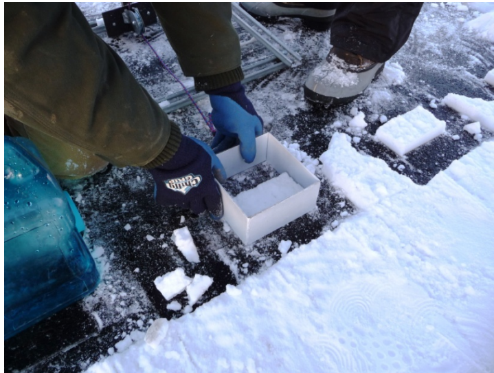
Figure 36. Measuring bond shear strength during Field Test III with the new plow box.
