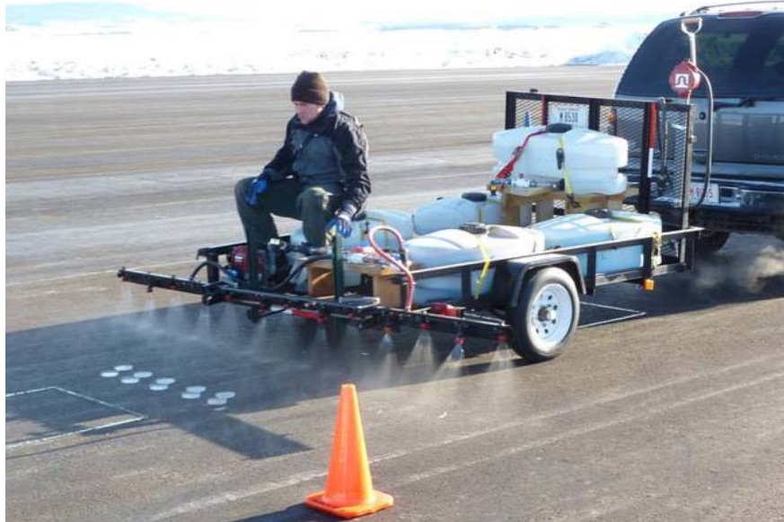
Figure 33: Applying chemical to a test section with the anti-icing trailer.
