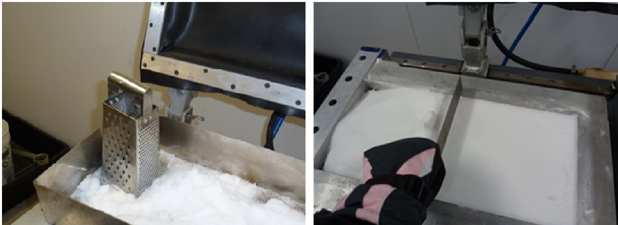
Figure 7: Grated snow is sieved onto the pavement sample (left) and leveled with a screed (right).
