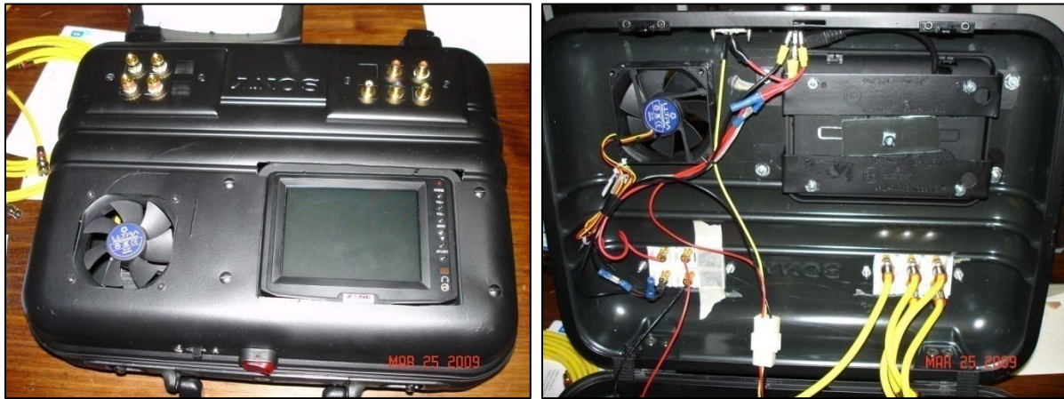
Figure 4-8. DAS unit outside and inside
