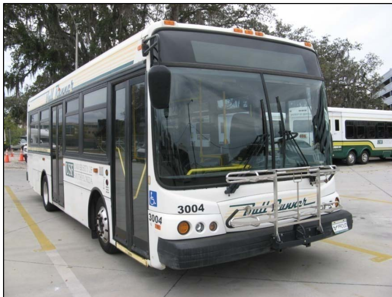
Figure 3-2. Ultra-low floor bus
