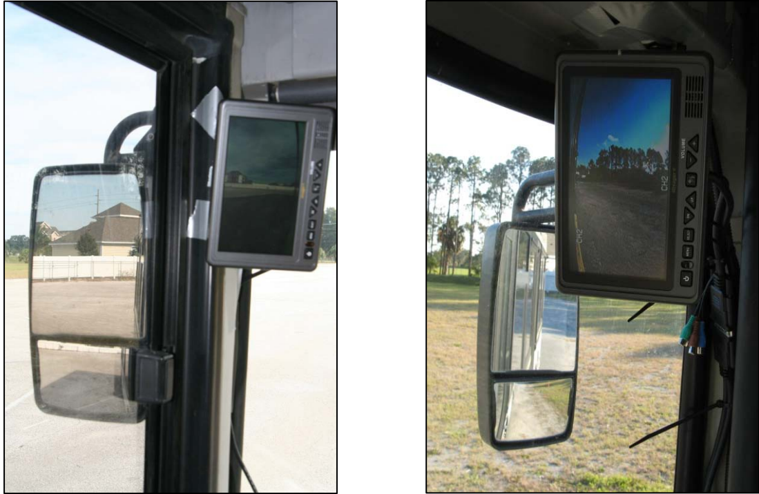
Figure 5-24. Left and right monitor installed next to mirror in portrait orientation
