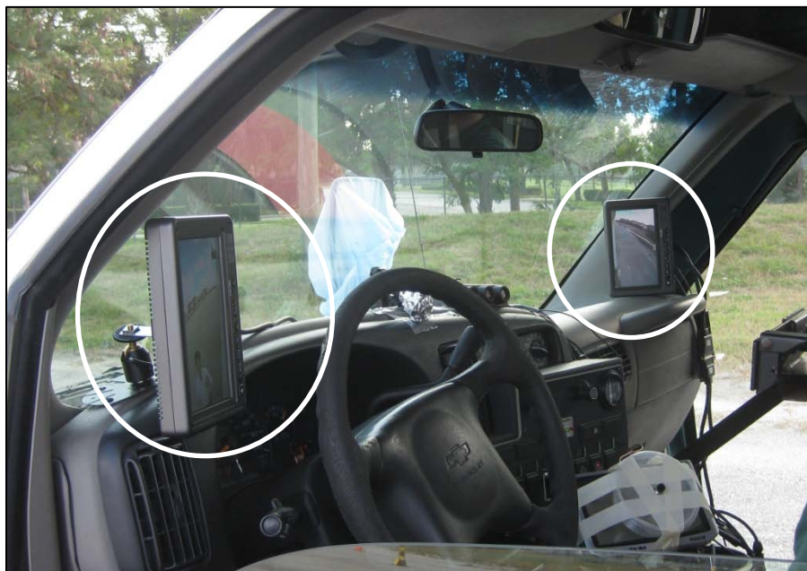
Figure 2-8. Two monitors installed on driver's dashboard
