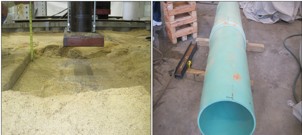
Figure 52. Visual Inspection of Jointed PVC Pipe after Fatigue Test.
