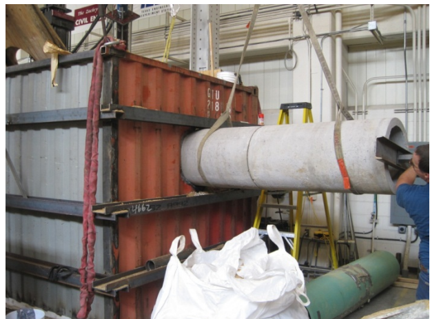
Step 6. Install pipe after instrumentation.
