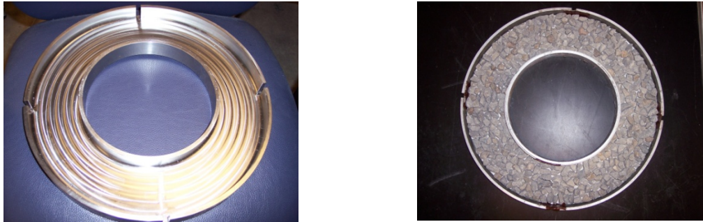
Figure 1. Casting mold and specimen coupon.
