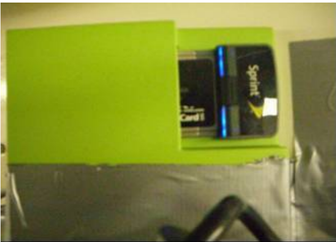
Figure 29: Junxion EV-DO Router for Pelco Camera
