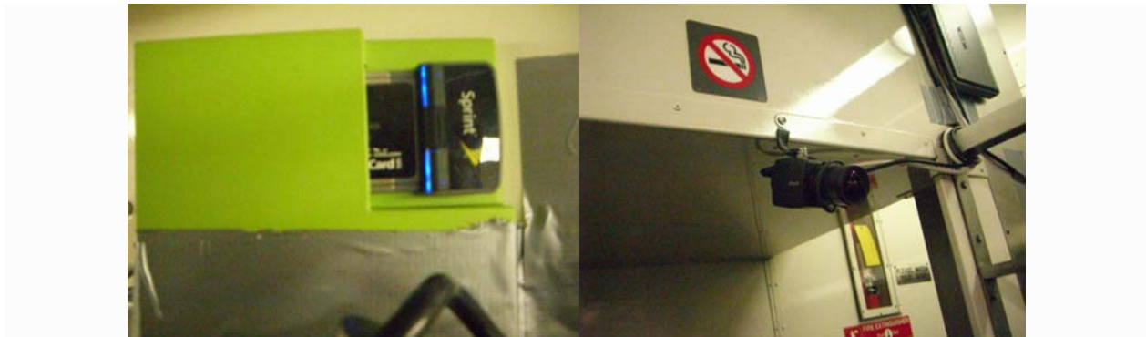
Figure 6: EV-DO Router and Camera - Passenger Car
