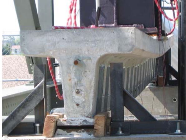
FIGURE 5.40. Beam 5 during loading.
