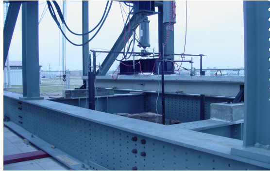
FIGURE 3.6. Beam in test frame.
