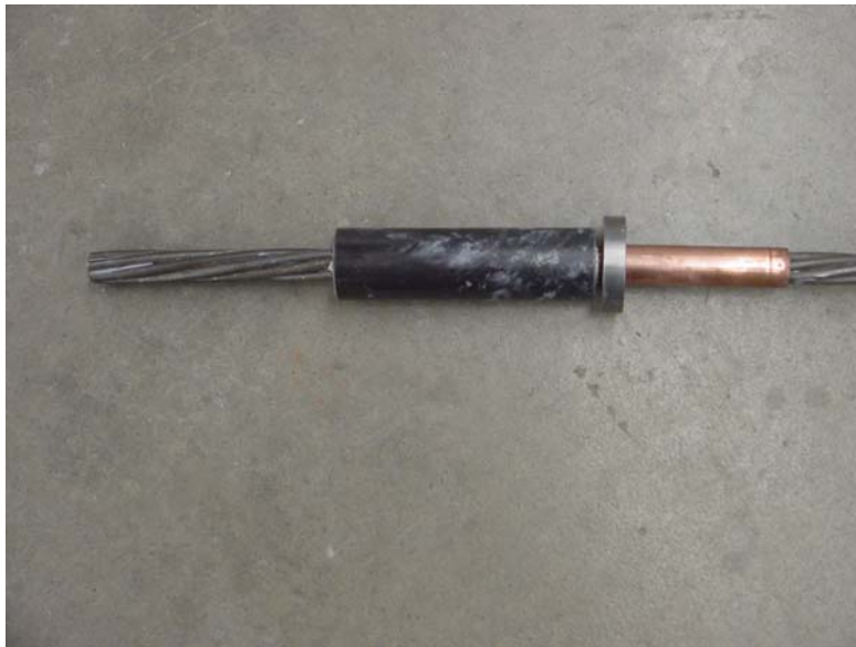
FIGURE 5.65. Embedding prestressing strand end through epoxy-filled thick metal cylinder grip.
