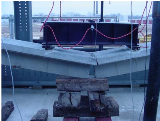
FIGURE 5.6. Failure configuration of control beam.
