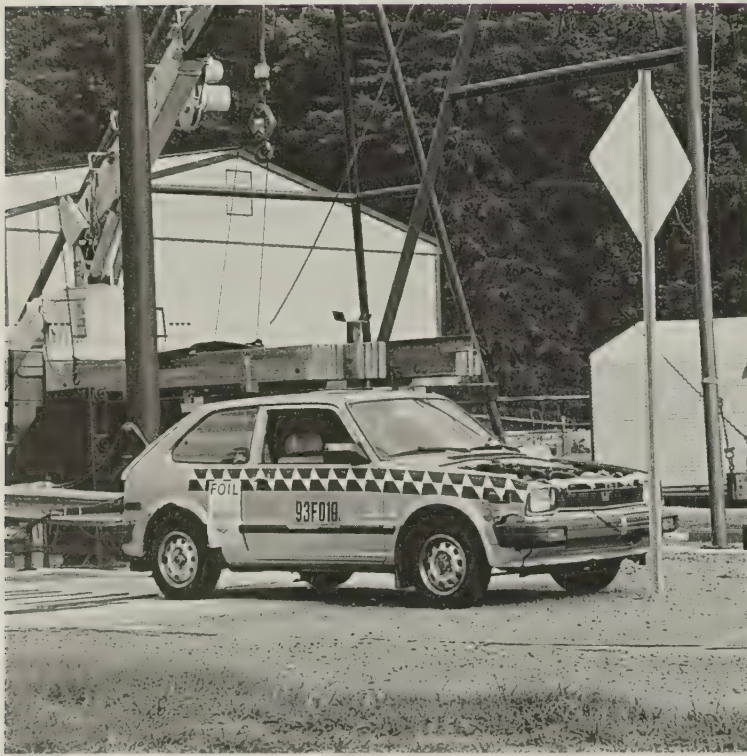
Figure 1—Photograph and corresponding finite element model of the pre-collision with a sign post.
