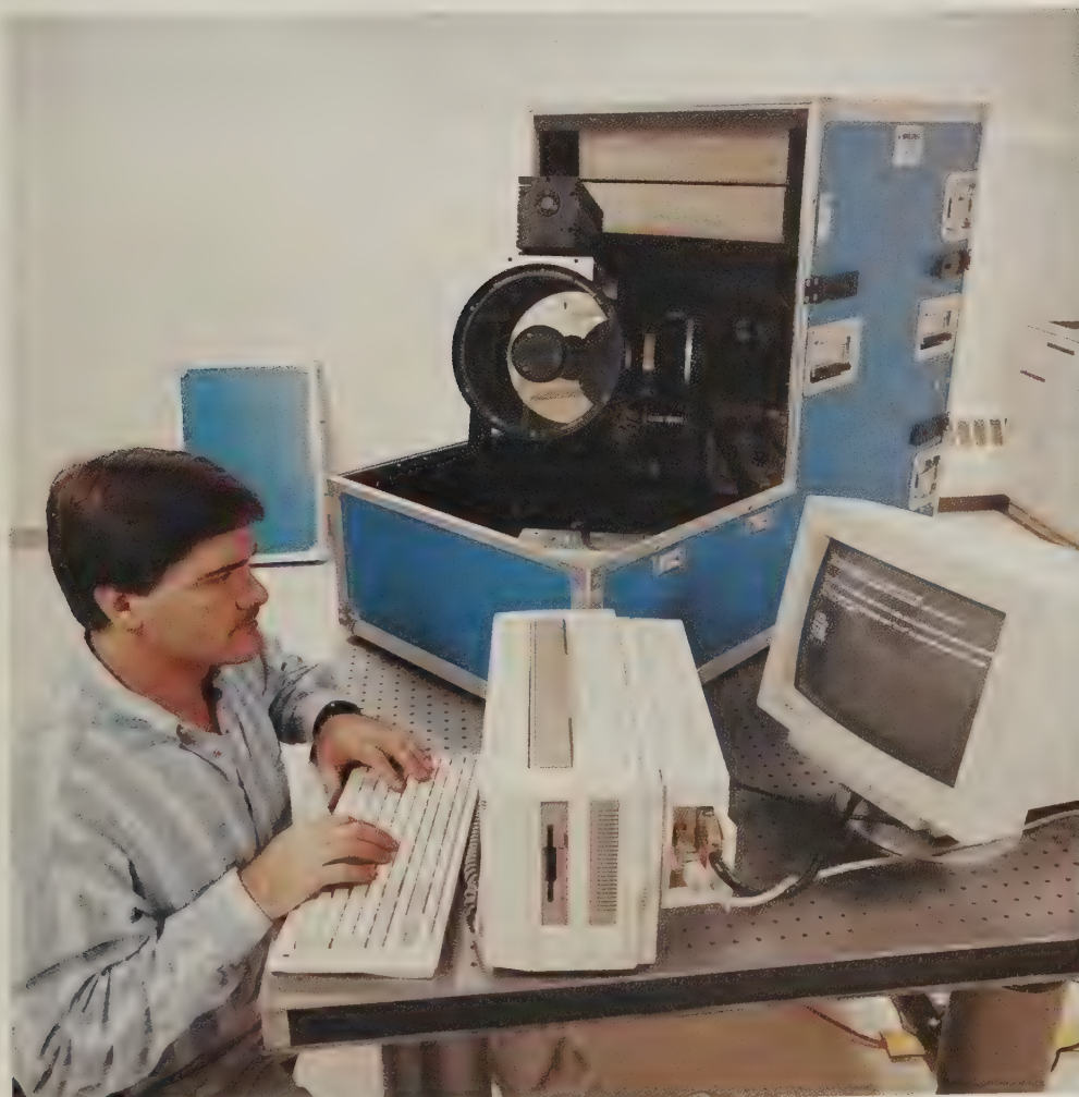
Locker-sized LIDAR equipment used in the Barcelona air quality measurements.
