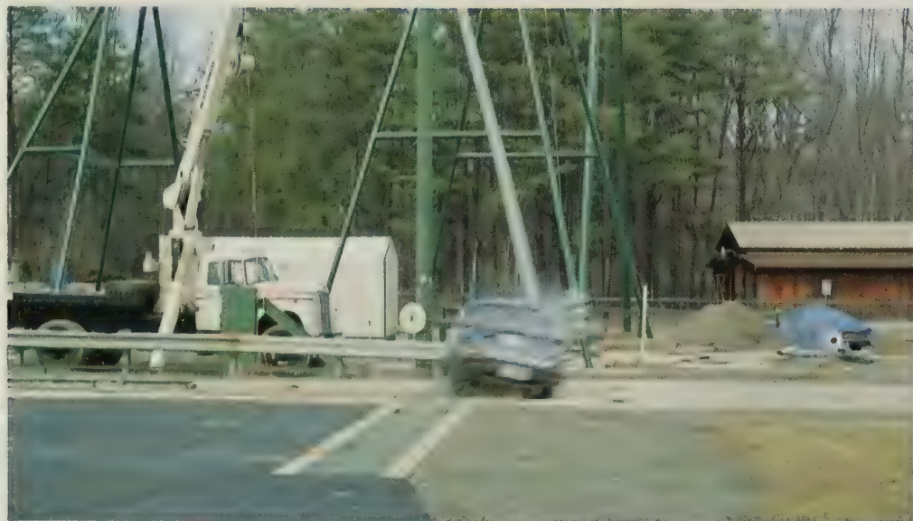
At the Federal Outdoor Impact Laboratory, a car is crashed into a guardrail terminal as part of a series of tests on side impacts.
