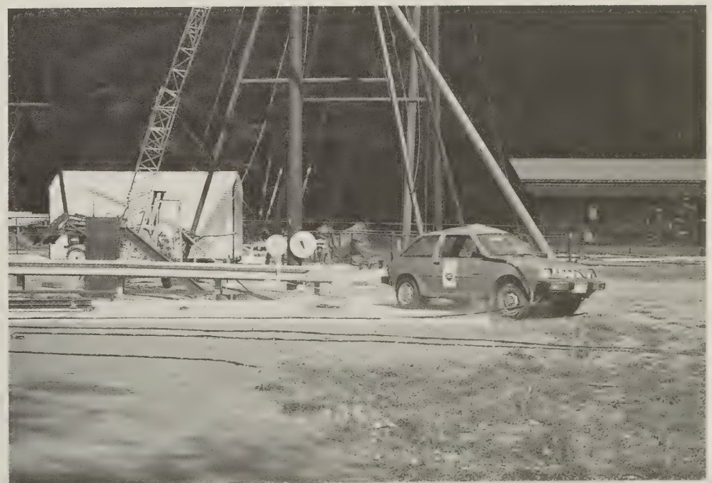
Side impact into a utility pole was part of the FOIL testing.
