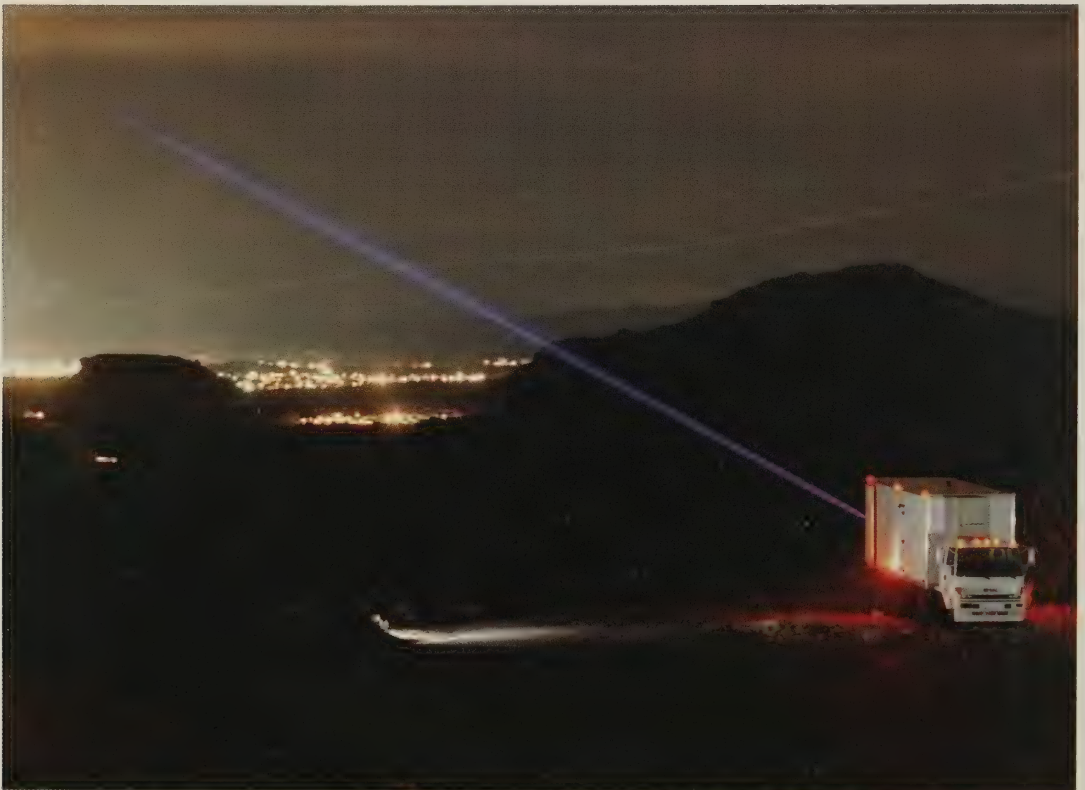
LIDAR laser beam reaching out over a region of Mexico City to document air pollution sources.
