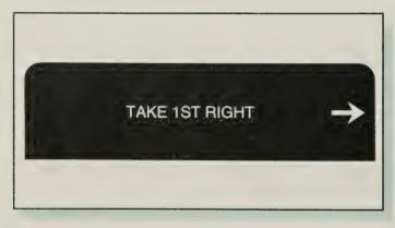
Figure 2.—Sketch of medium visual guidance unit display.
