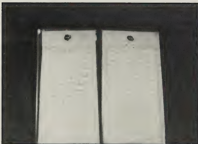
Figure 10.—Condition of CALTRANS water-borne acrylic system after 1,500 hours of UV/condensation exposure.
