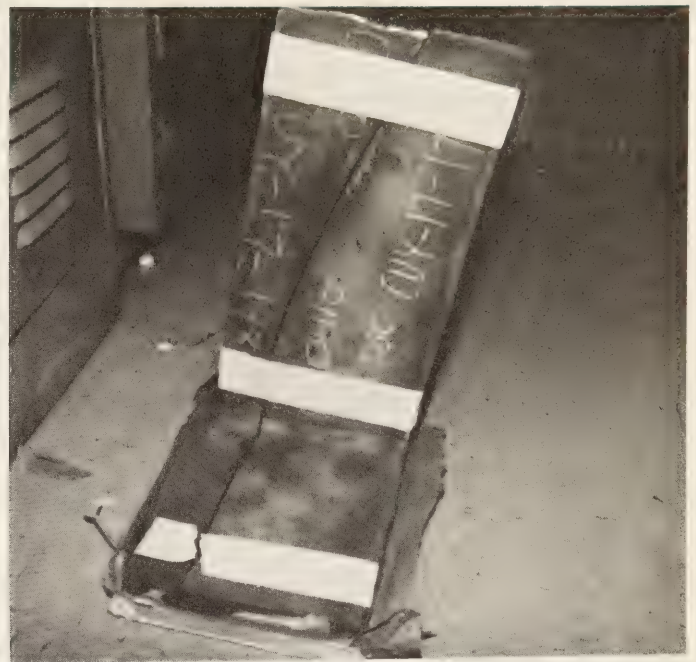
Figure 4.—Cracked section as received in the laboratory.
