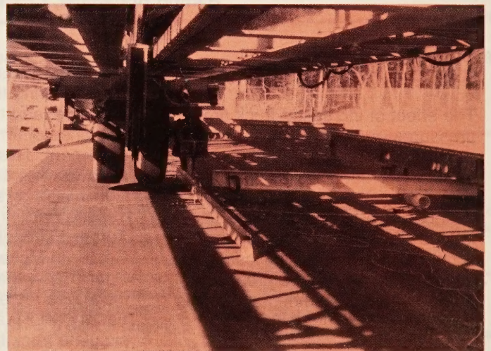
Figure 2.—ALF dual wheel assembly and pavement instrumentation.
