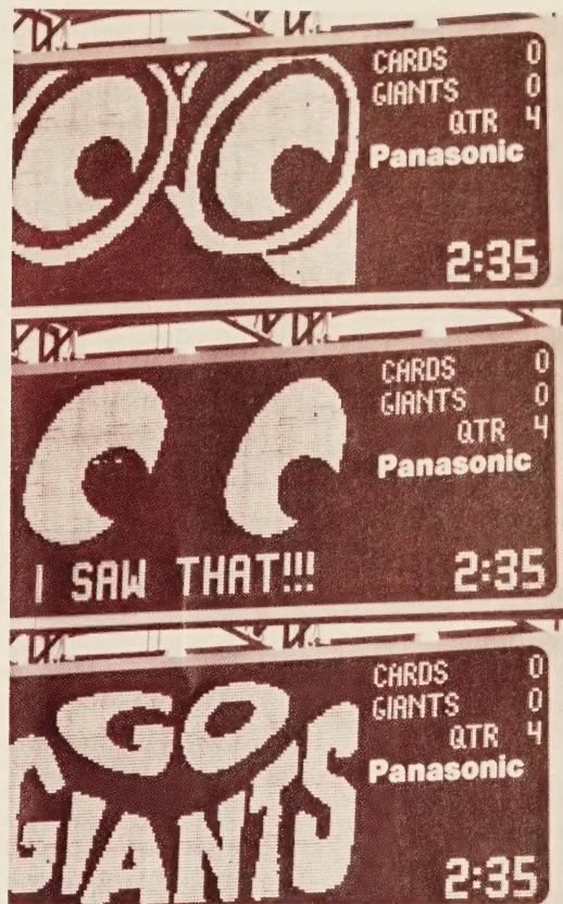
Figure 2.—A remotely controlled lamp matrix scoreboard.
