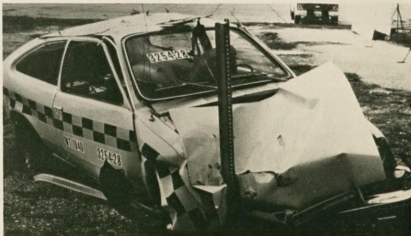
Figure 16.—Test results of 0.88 Mg (1,940 lb) vehicle traveling 97 km/h (60 mph).
