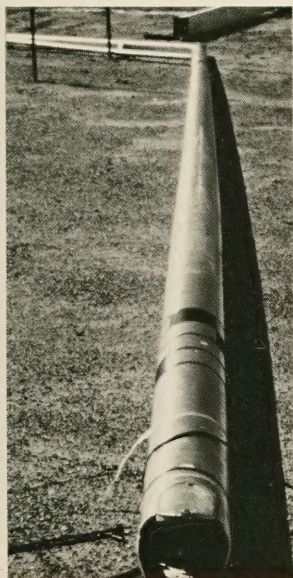
Figure 3.—A luminaire support used to test the impact with a 1.63 Mg (3,600 lb) vehicle traveling 64 km/h (40 mph).
