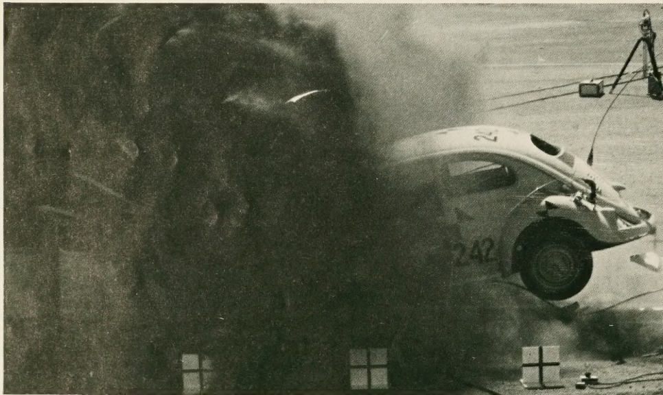
Figure 6.—An impact attenuator test—an 0.88 Mg (1,940 lb) vehicle traveling 95 km/h (59 mph).
