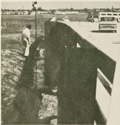
Figure 14.—Test results of 18.14 Mg (40,000 lb) bus traveling 89 km/h (55 mph), with an impact angle of 15°.
