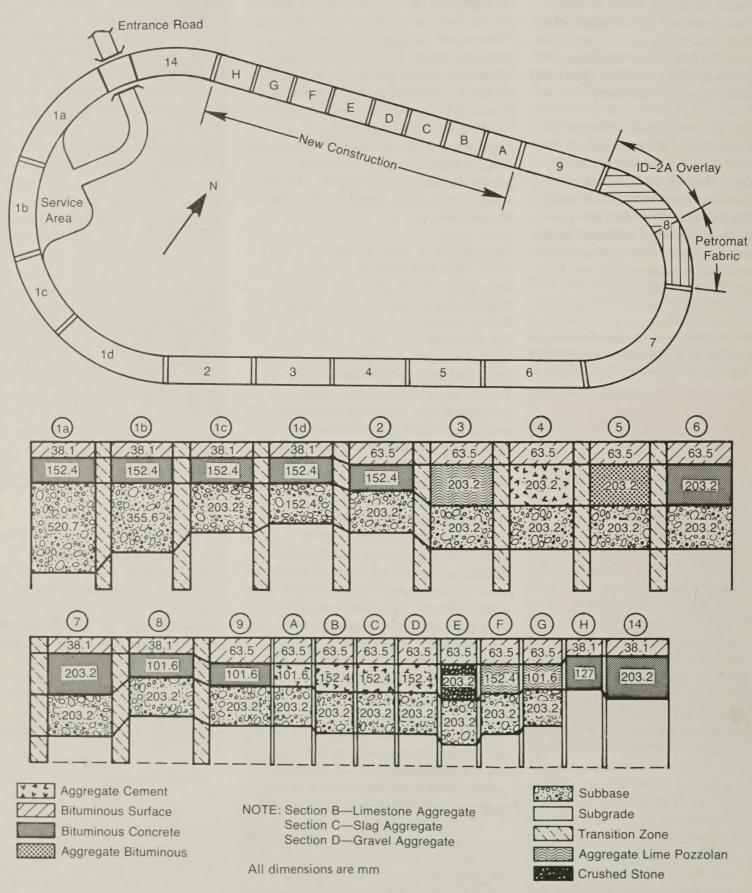
Figure 5. — Schematic of Pennsylvania State University test track.
