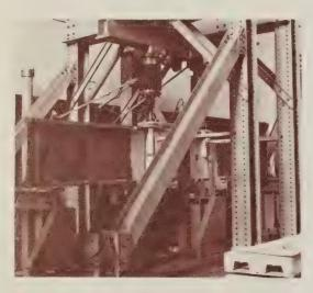
Determination of Tolerable Flaw Sizes in Full-Size Welded Bridge Details, Report No. FHWA-RD-77-170
