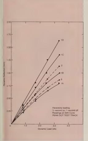
Figure 6. — Results from the Pennsylvania State University testing.
