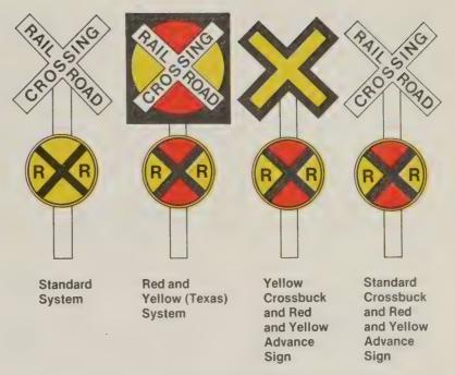
Figure 1.—Crossbucks and advance warning signs tested in Phase 2.
