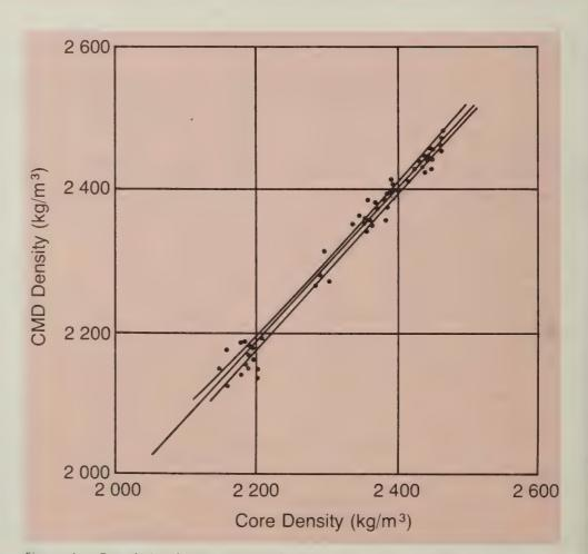
Figure 4.—Correlation between CMD density and core density measurements, laboratory static and dynamic tests (regression line and 95 percent confidence limits).
