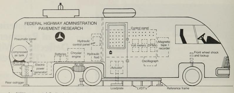
Figure 1. —FHWA pavement deflection test system.
