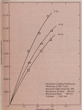
cooperation with the Maryland Department of Transportation and the University of Maryland, is using "Thumper" to get deflection measurements at various sites in Maryland under differing seasonal climatic conditions. The objective is to use the capabilities of the device in developing a standard nondestructive method of measuring the stiffness properties of the pavement system for use in a layered system computer program for design of overlays.
