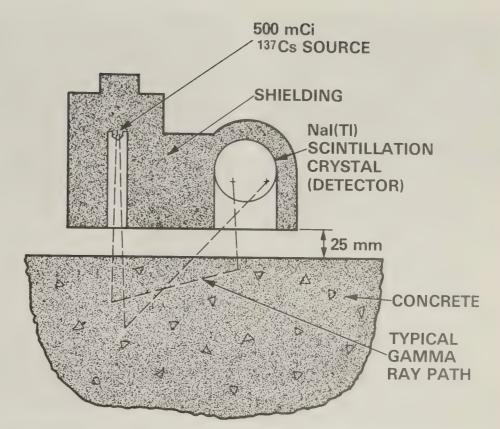
Figure 1.—Backscatter measurement with CMD source/sensor unit.
