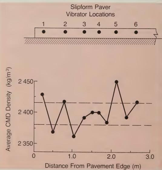
the pavement surface at speeds up to 0.085 m/s. The device can duplicate core density measurements within a 35 kg/m<sup>3</sup> confidence range (95 percent confidence limits).
